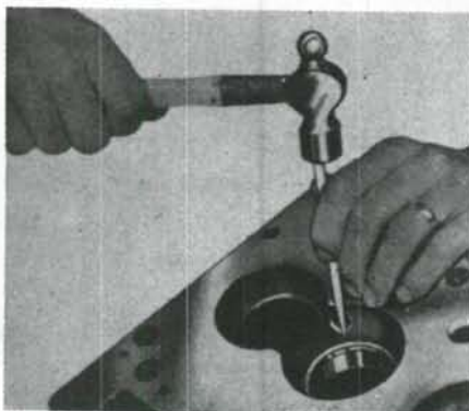
Fig. AC55—Method of removing a valve seat insert.
