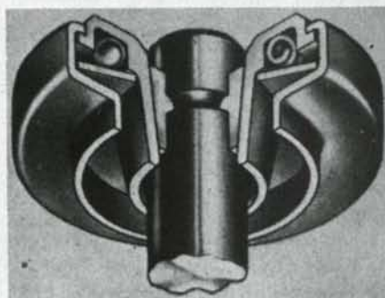
Fig. AC23—WD engines after engine serial 299173, and engines 262650 through 263224 and WD45 are factory equipped with Rotocap positive type valve rotators for the exhaust valves. Rotators are also available for service on the WC and WF engines.
