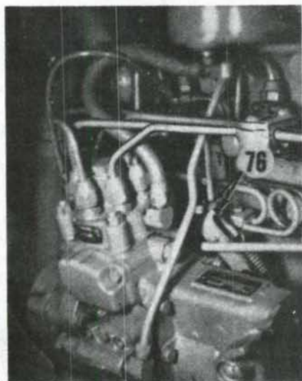
Fig. AC66 — The engine high idle speed is adjusted with nuts (76).
