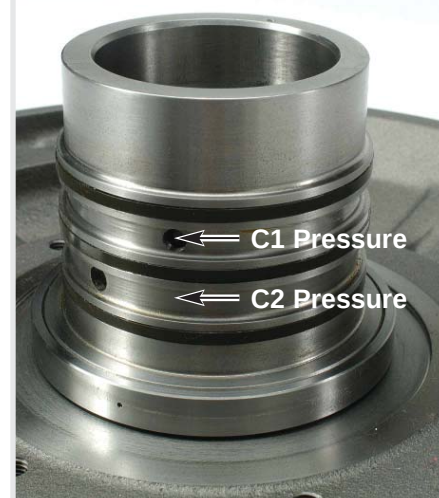
Front support oil passage detail - outside hub.
