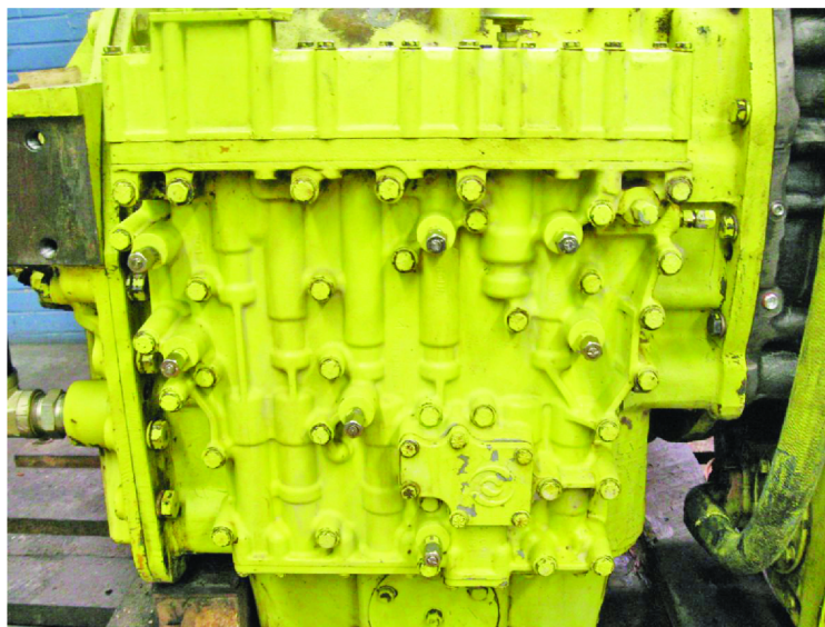
Figure 2. Identification of Control Valve Body with Contoured Valve Body Casting
