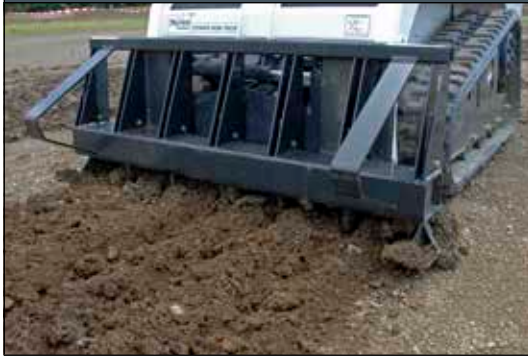
Scarifier: Includes 2 Depth Guides and 5 teeth.
