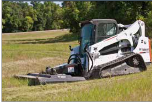
Brushcat™ Rotary Cutter: Comes standard with a 7 cm Offset Blade and Front Wheels. Cutting height of 5 cm.
