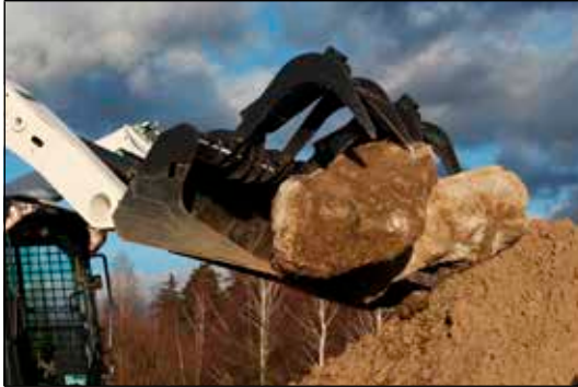
Bucket Grapples: Includes Bolt-On Cutting Edge.
