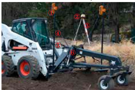
Grader 213 cm with Laser Equipment
