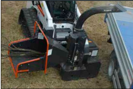
Wood Chipper: Loader must be equipped with a 7-Pin Control Kit.
