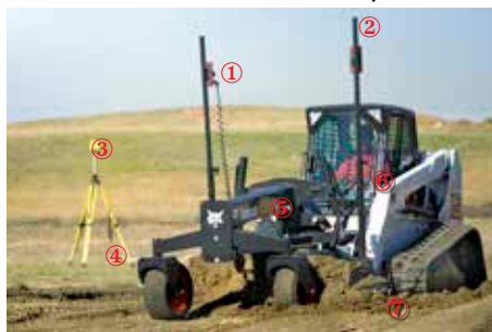
Grader 244 cm and 274 cm with Laser System
