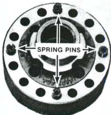
Fig. 24—Install double spring pins in differential case half as shown. Refer to text.
