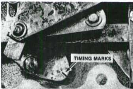
Fig. 268—Timing marks in linkage box should align as shown. Refer to text.
