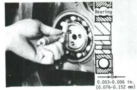
Fig. 105—View showing measurement of intermediate shaft recess from bearing face to determine shim pack. Refer to text.
