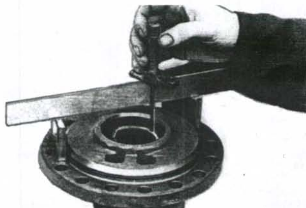
Fig. 21—Measure distance between right axle housing flange and bearing cup seat (shoulder).
