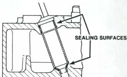
Fig. 47—Apply Grade B Loctite to sealing surfaces of nozzle sleeve.
