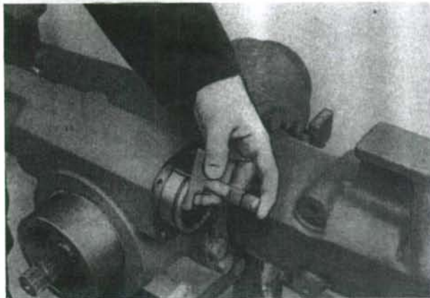
Fig. 43—Using a depth gage, measure distance between axle housing and end of cylinder sleeve. Refer to text.
