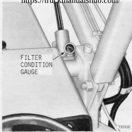
Figure 65 - Filter Condition Gauge
