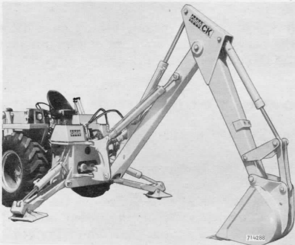
Figure 41 - Backhoe In Tripod Position
