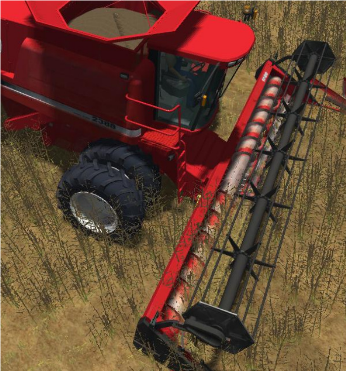
Figure 22: A slugged header will cause you to miss spots. Reverse the combine to clear the slug
