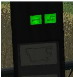
Figure 7: The pipe out and unloading indication lights
