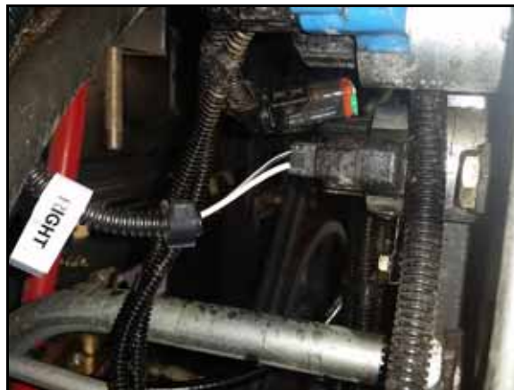
FIGURE 14. RIGHT Valve Harness Connector Installed
