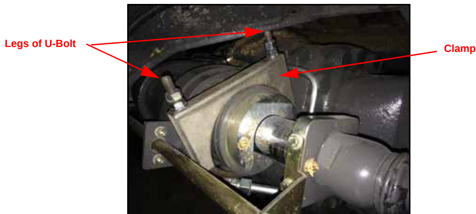
FIGURE 4. Muffler Clamp Installed on Steering Cylinder Barrel
