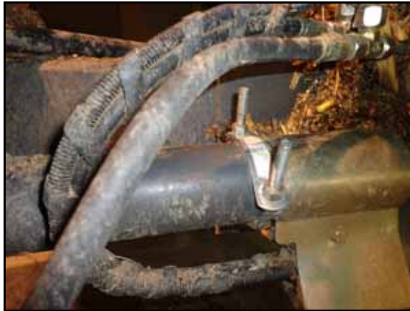
FIGURE 10. Large Muffler Clamp Installed
