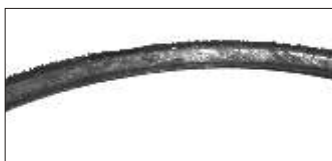
Shining surface due to high slippage
