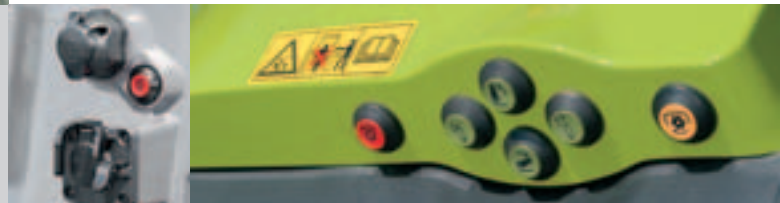
External controls for front and rear PTO
