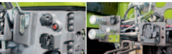
ISOBUS connections at the front and rear
