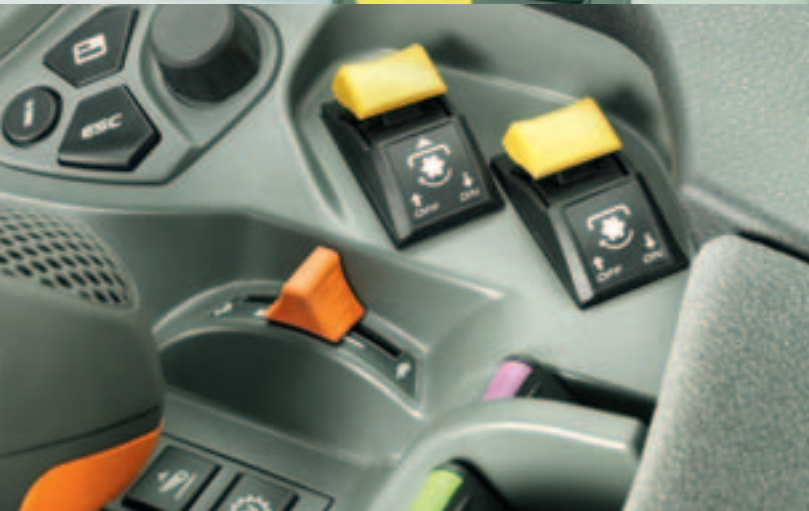
External controls for front and rear PTO
