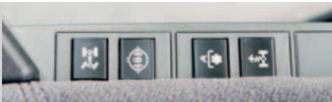
Control panel (11) in the armrest: four-wheel drive, differential lock, automatic PTO engagement/disengagement and front axle suspension
