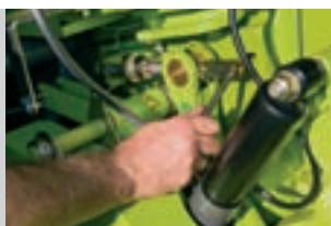
Mechanical shear bar adjustment
