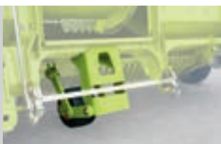
Support wheel for optimal ground-contour following
