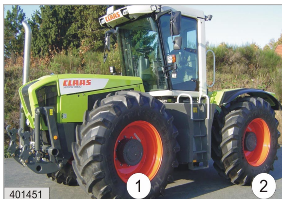
1 = Floating axle 2 = Rigid axle
