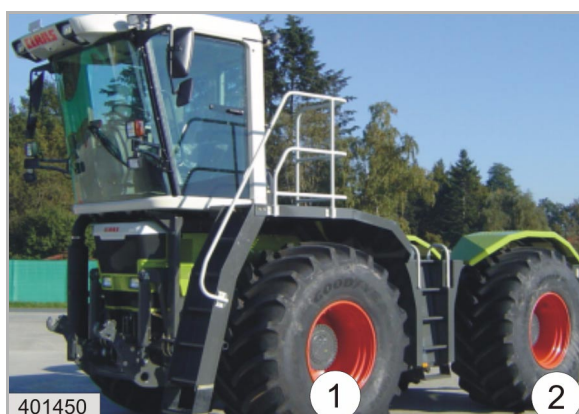
1 = Floating axle 2 = Rigid axle
