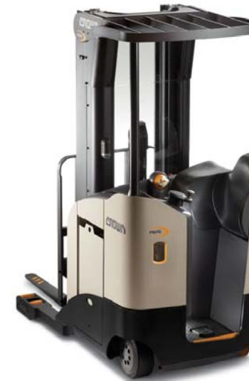
RR 5715 – 24 volt – 42-in power unit – Max lift height = 270 in
