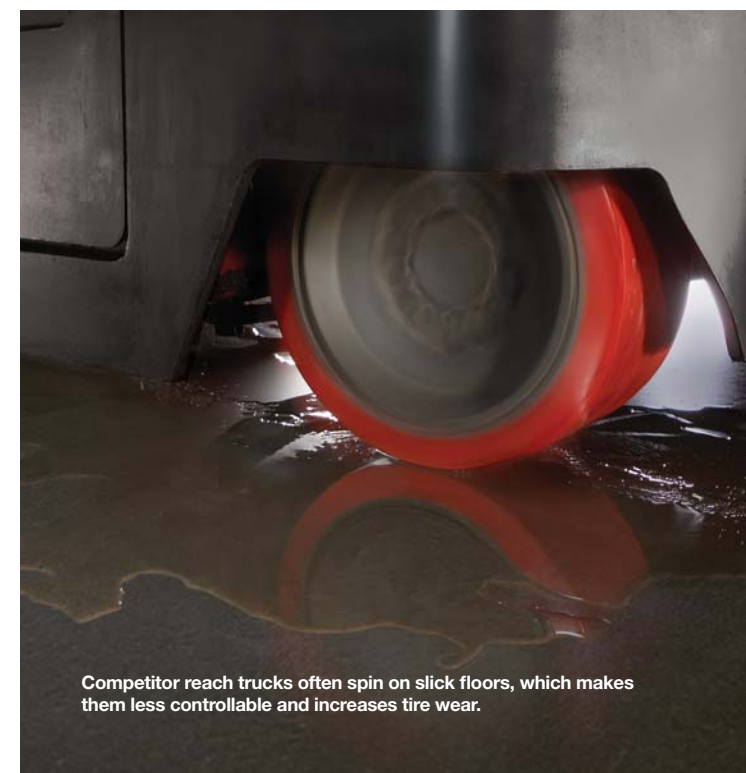
OnTrac™ Anti-Slip Traction Control reduces tire spin and provides maximum available traction during acceleration, plugging and braking by monitoring changing conditions.
