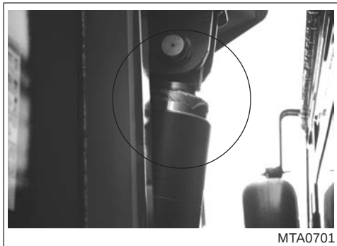
(2) Incorrect position of cylinder tube(1st stage tube protruded)
