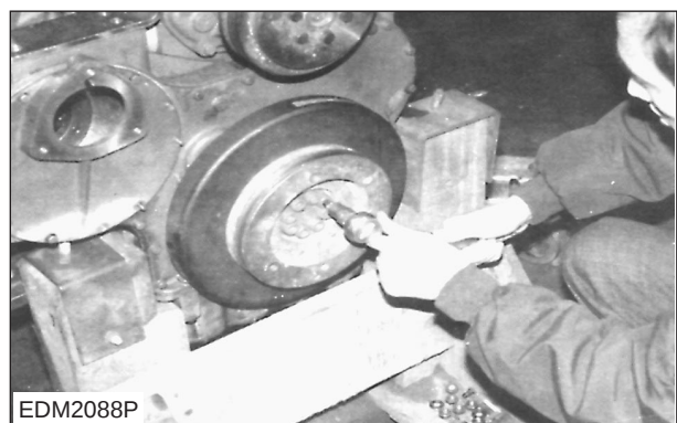
<Fig.94> Vibration Damper Assembling
