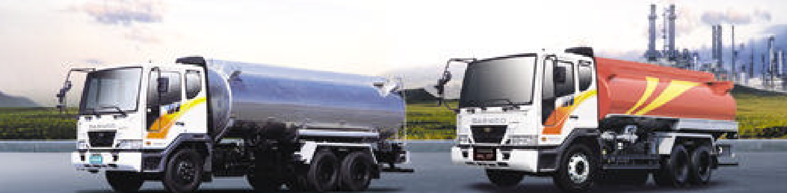
Twin-chamber design facilitates loading and delivery from either right or side.
