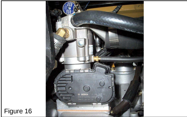
(Figure 16) shows the N-CA55-500TR mixer installed with the electronic throttle.
