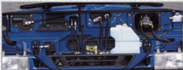
Lockable front panel Facilitates repairs and maintenance without tilting cab
