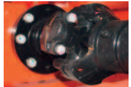
Propeller shaft. A protective cover has been installed to protect the oil seal from dust, foreign objects and premature wear.
