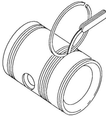
Figure 23. Measuring Piston Ring Side Clearance
