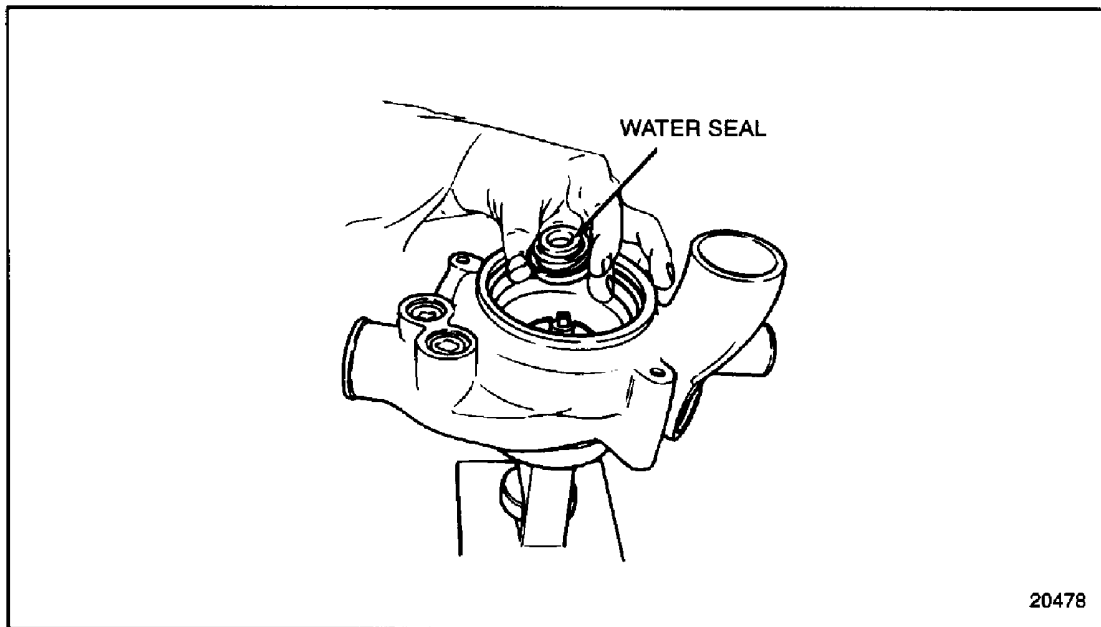
Figure 4-24 Water Seal Insertion
