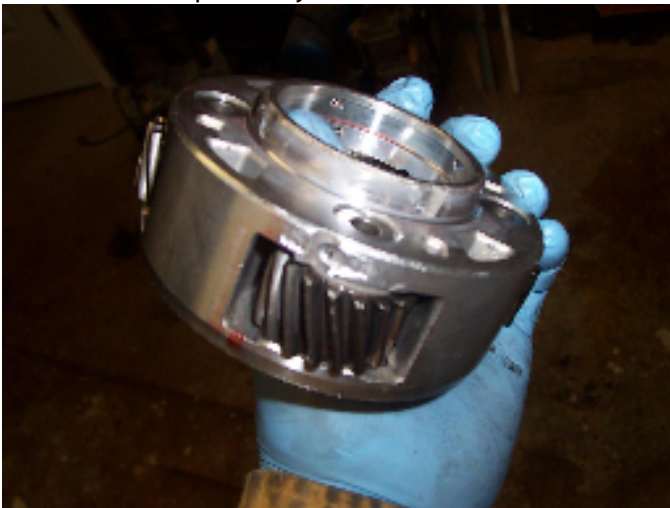
6. Front view of planetary. Check for wobble of the planetary gears.
