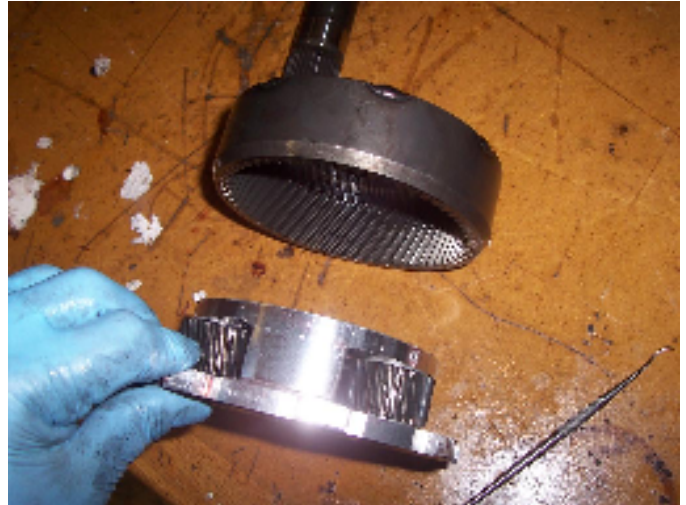
11. Planetary and annulus gear separated
