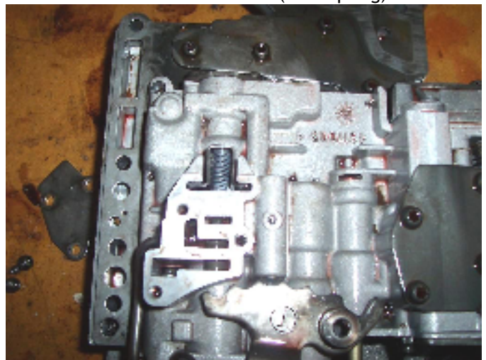
10. Boost Valve Cover Removed (note spring)
