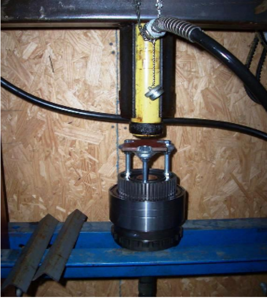
8. OD unit in a press getting ready to remove the snap rings that hold the 800lb spring
