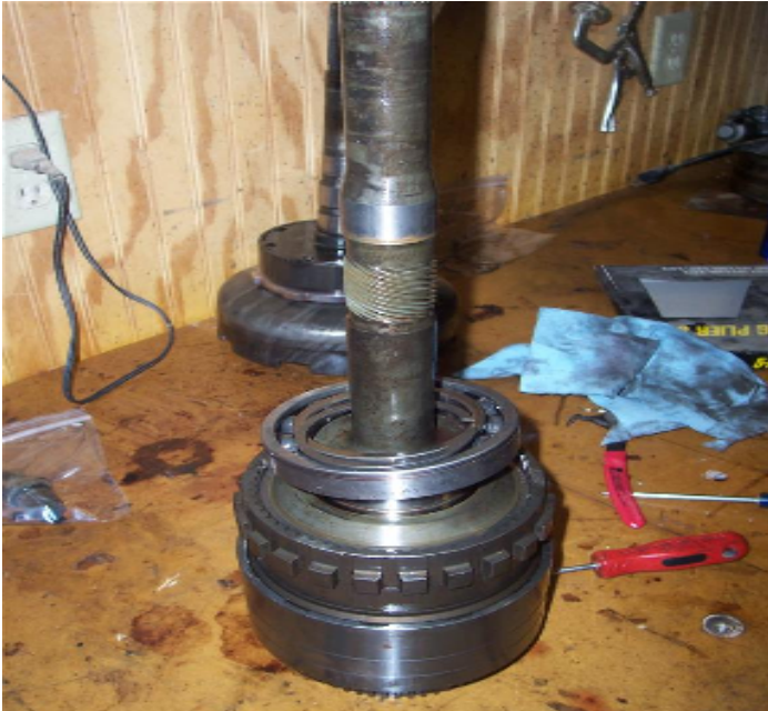
6. OD assembly that is inside the OD unit case. This is the assembly that has the 800 pound spring in it.
