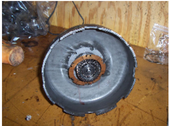
7. The driving shell after the planetary has been removed.
