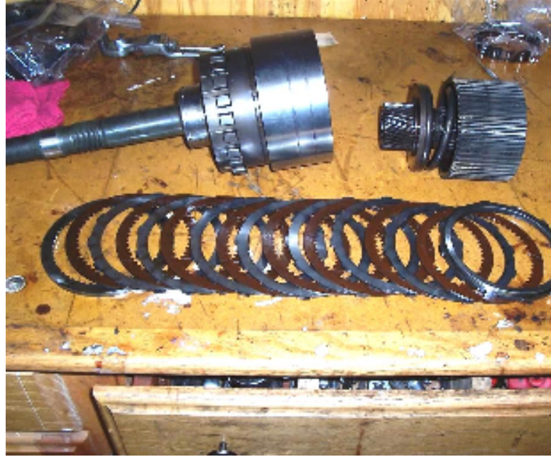
10. OD clutch pack underneath the 800lb spring. The clutches go inside the shell you see up top.
