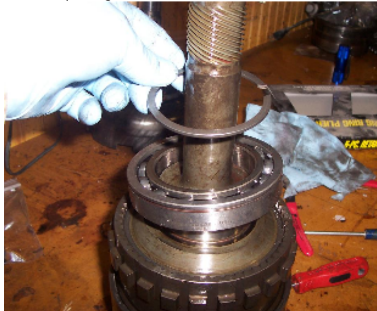
7. Back end of OD unit, showing rear bearing and snap ring. The shaft you see is what actually exits from the rear of the tranny. The worm gear at the top of the pic is for the speedo gear.
