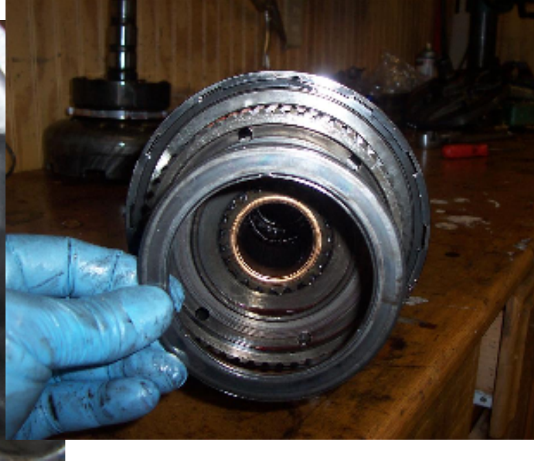
6. Overdrive thrust bearing which rides on top of the huge annulus gear
