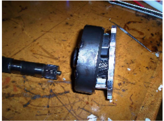
11. Planetary and annulus gear separated
