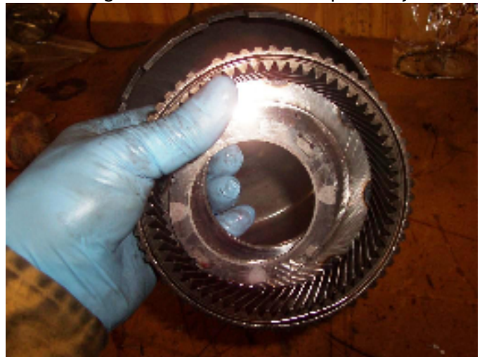
7. The driving shell after the planetary has been removed.
