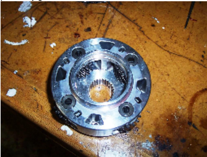
6. Front view of planetary. Check for wobble of the planetary gears.
