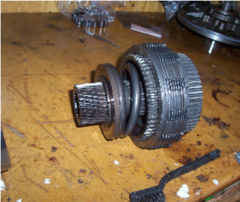
9. Post spring removal. The rear of the annulus gear with the 800lb spring exposed and sungear.
