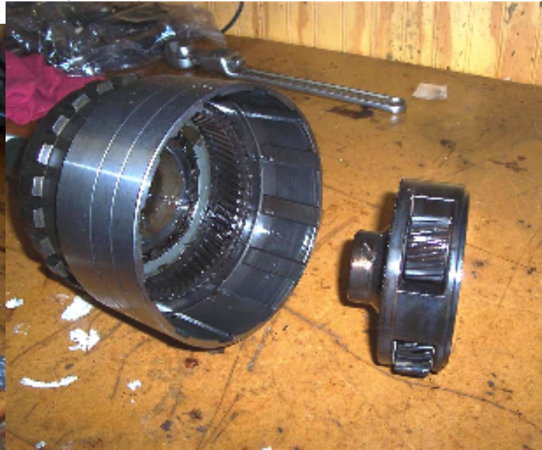
11. OD planetary that sits underneath the clutch pack.
