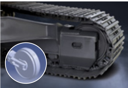
Integrated Track Spring and Idler The track spring and the idler have been joined directly to achieve high durability and improved maintenance convenience.
