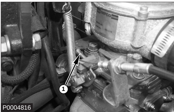
Low Idle Speed Adjustment (1) Idle speed screw.
