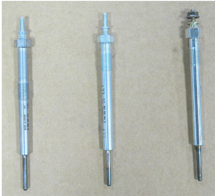
Figure 11. The glow plug on the left is for the early production injector under cover cylinder head. The center one came on the scene in mid '04 MY and is used through '05 MY and the last one on the right is '06 MY through current production. They are all different and do not interchange.
