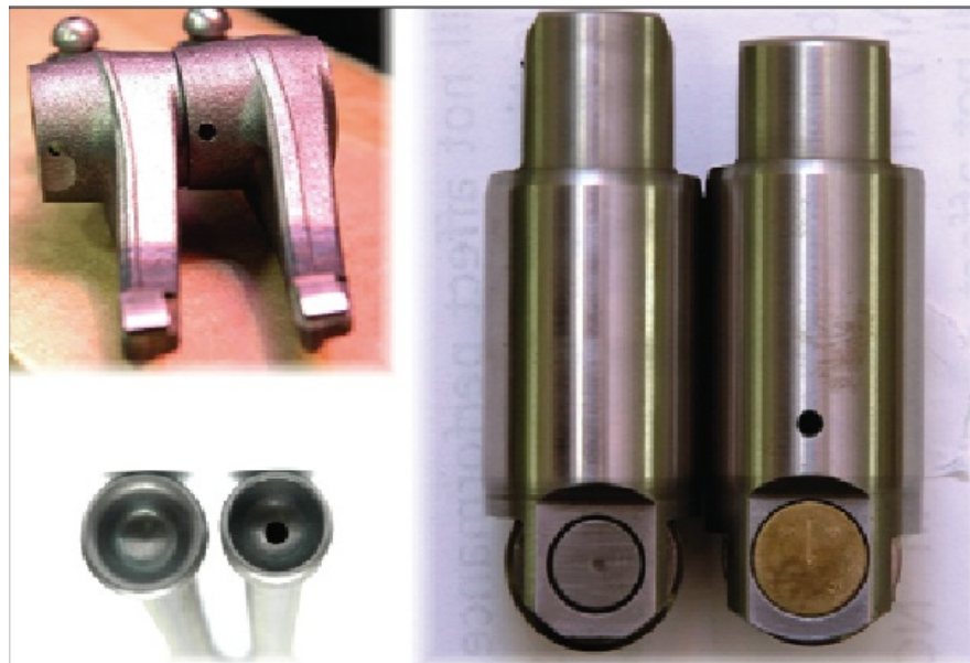
Figure 5. The upper left has the '05 MY on the left and '06 MY on right – note the difference in oil hole size. Pushrods on the lower left are '05 MY and earlier on the left and '06 MY and later on the right. Lastly, on the right side of the picture, the cam follower on the left is through '05 MY and '06 MY to current is on the right.
