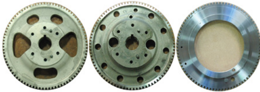
Figure 4. Camshaft timing gear on the left is early solid style thru '05 MY and on right the two pieces that are used as the spring loaded assembly to avoid and eliminate potential timing noise '06 MY to current.
