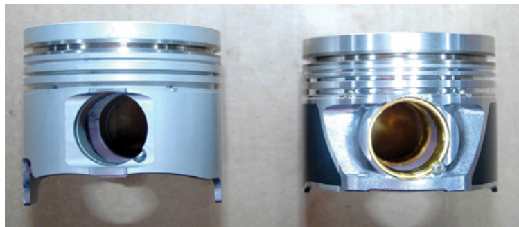
Figure 6. The piston on left was used up through the '05 MY and the piston on right is '06 MY and later with a longer wrist pin.
