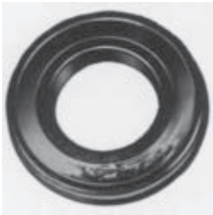
Bearing removed with punch, damaged shield.
