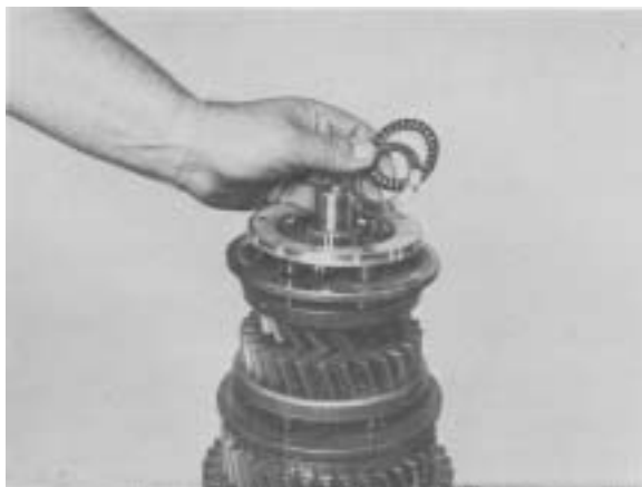
Figure 19 - Remove shift hub thrust bearing and bearing race.
