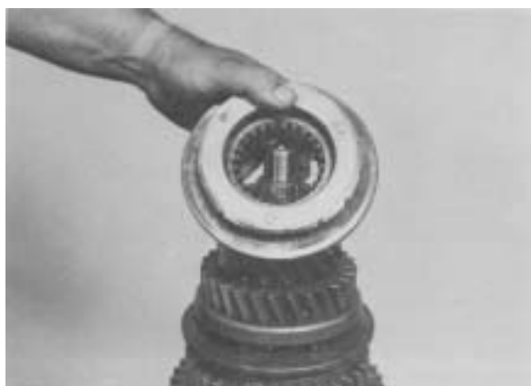
Figure 20 - Remove 4th & 5th speed synchronizer assembly/
