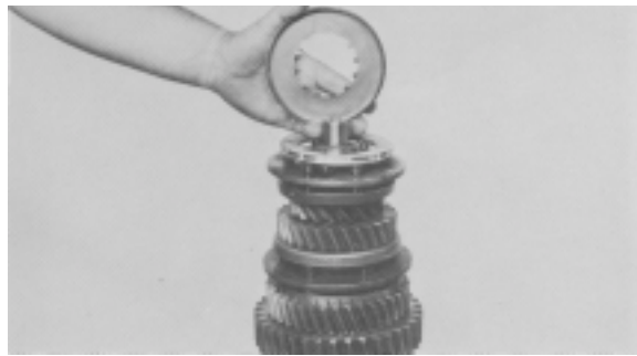
Figure 18 - Remove 5th-Speed synchronizer cup.
