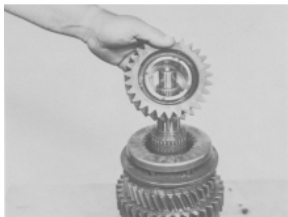
Figure 26 - Remove 3rd speed gear.
