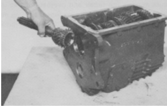
Figure 7 - Remove main drive gear and bearing assembly.
