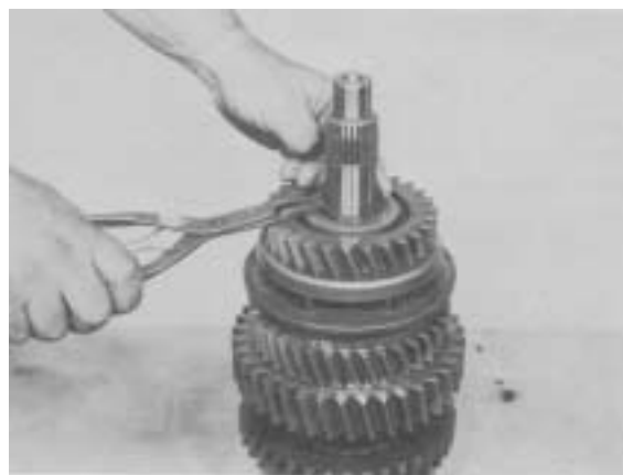
Figure 24 - Remove 3rd gear locating washer retaining ring.
