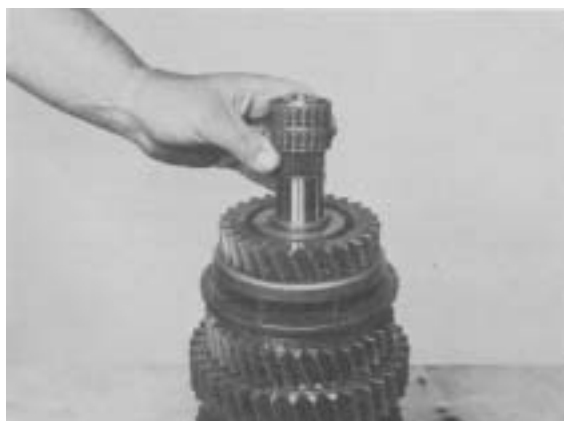
Figure 23 - Remove 4th gear bearing.
