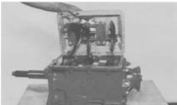
Figure 2 - Remove control cover assembly.
