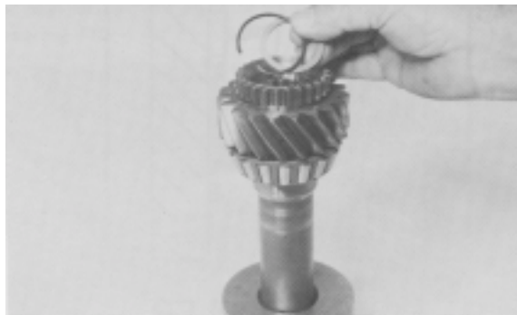
Figure 88 - Install roller bearing washer and retainer ring.
