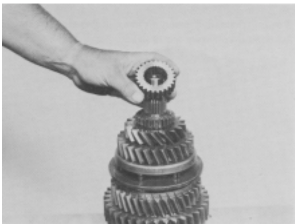
Figure 21 - Remove the 4th & 5th shift hub sleeve.
