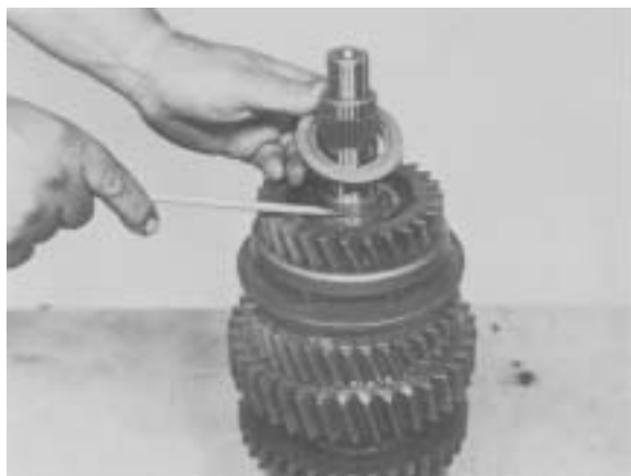
Figure 25 - Remove washer and lock ball.
