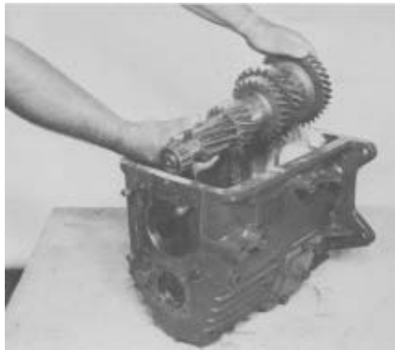
Figure 12 - Remove countershaft assembly.
