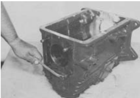
Figure 9 - Remove countershaft bearing cap bolts.
