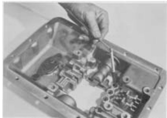
Figure 115 - Remove poppet springs, quantity 4.
