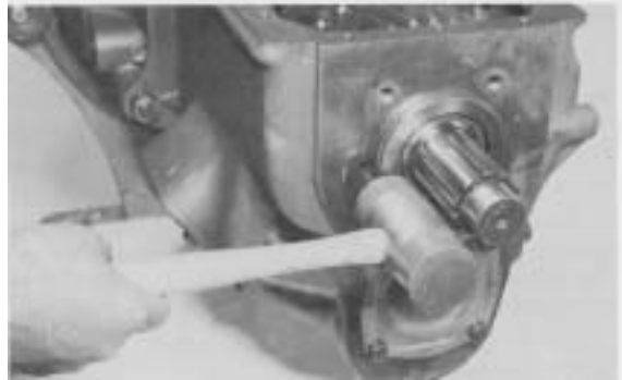
Figure 154 - Using a soft hammer, tap rear bearing cup until cup locating ring is against housing.
