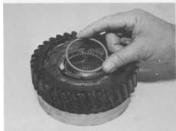
Figure 49 - Position outer roller spacer on second row of rollers. Grease rollers to hold in place.
