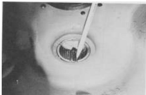
Figure 138 - Coat countershaft pilot bearing needle rollers with heavy grease to hold in place until countershaft is installed.
