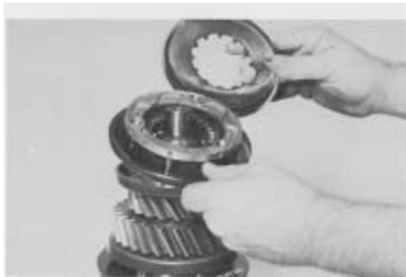
Figure 19 - Remove 5th speed synchronizer cup and 4th & 5th speed synchronizer assembly.
