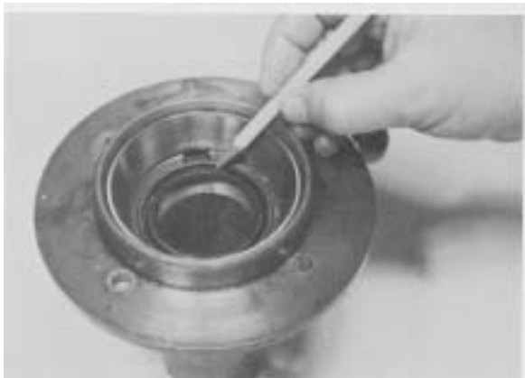
Figure 158 - Coat O.D. of oil seal with Loctite 510 and install with lip of seal up in main drive gear bearing cap.
