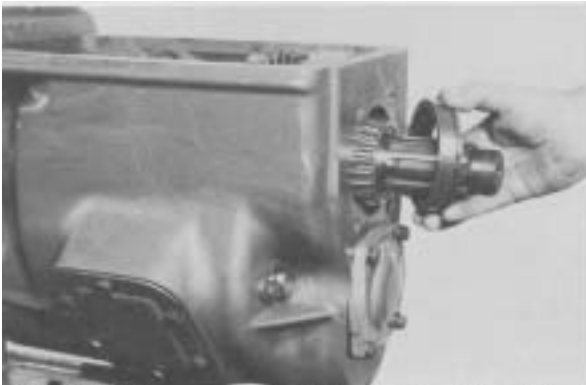
Figure 153 - Position mainshaft rear bearing cup in housing bore.
