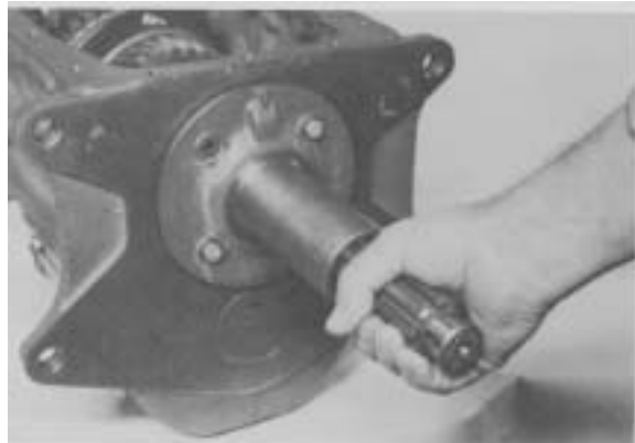
Figure 161 - Turn main drive gear and mainshaft by hand back and forth to seat taper bearings.
