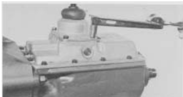
Figure 169 - With special shift lever control top gasket in position install control top or remote control assembly on control cover. Tighten screws 20 - 25 ft. lbs. torque [27,1 - 33,8 N.m].
