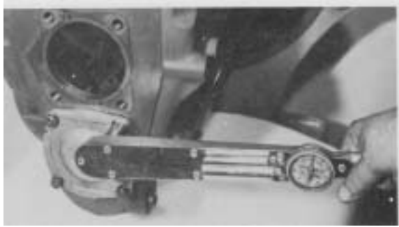
Figure 151 - Coat a new gasket on both sides with Loctite 510. Position gasket on countershaft bearing cap. Install bearing cap and bolts. Tighten bolts 20 - 25 ft.lbs. torque [27,2 - 33,8 N.m.]
