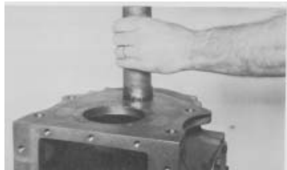
Figure 81 - If countershaft front bearing is to be replaced, remove clutch housing and drive front bearing from transmission case. Apply a light coat of Loctite 510 on the outer diameter of the new bearing. Install in transmission case as shown with end of bearing .001-.007 below the face of case. Clutch housing is reassembled temporarily on transmission to facilitate reassembly of transmission, but will be removed again later on to set mainshaft taper bearing end play.
