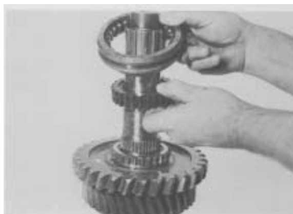
Figure 33 - Remove shift hub and sleeve.
