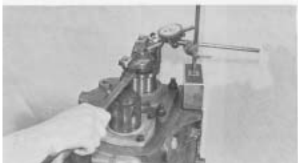
Figure 167 - Place transmission in vertical position, with main drive gear pointing down. Install transmission output flange and torque the nut. Roll main drive gear and mainshaft to seat front and rear taper bearings. Position a dial indicator as shown. Pry on output flange to get mainshaft end play. End play must be between .002 - .008 [0,05 - 0,02]. Add shims for more end play or remove shims for less end play. NOTE: Each time a change is made, retorque stud nuts and roll mainshaft. Apply Loctite 510 to both sides of each shim.
