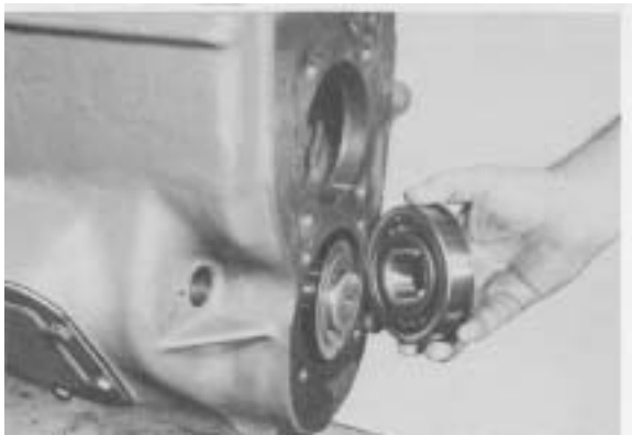
Figure 16 - Countershaft rear bearing removed. Note oil baffle position. Remove oil baffle.
