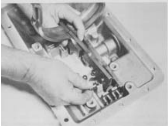
Figure 127 - Position 2nd & 3rd shift rail on poppet rail in neutral position with interlock pin aligned with 1st interlock tapered pin.
