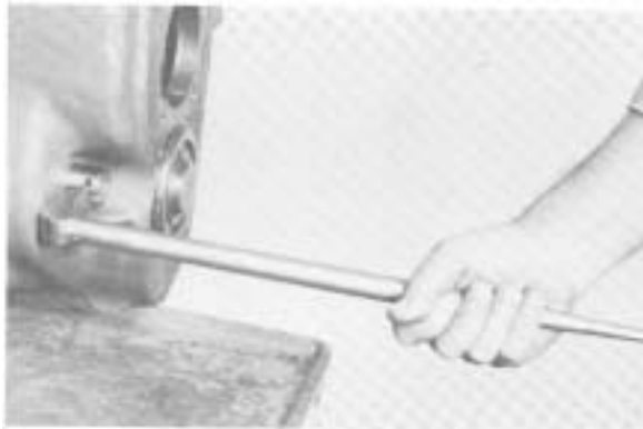
Figure 12 - Using a suitable puller, remove reverse idler shaft.
