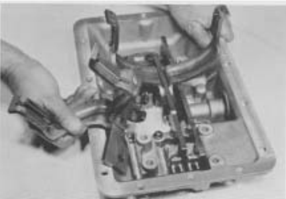
Figure 111 - Remove 4th, 5th, 2nd & 3rd shift fork and rail assembly (See caution in Figure 112).
