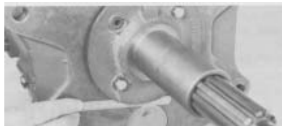
Figure 164 - Using taper gauge at other capscrew as shown. Record gap. Example: .037 [0,93 mm] average between one capscrew and the other would be .036 [0,91mm]. Using .036 as the average gap between the bearing cap and housing add .016 [0,40 mm]. Example .036 + .016 will give a shim pack of .052 [1,32 mm]. This shim pack example would give a mainshaft end play of .002 - .008 [0,051 - 0,203 mm].
