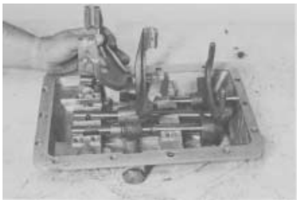
Figure 84 - Remove the 4th & 5th shift fork and rail assembly.
