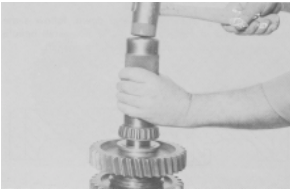
Figure 66 - Using a suitable bearing driver and soft hammer install mainshaft rear taper bearing. Be certain bearing race is tight against split washer.
