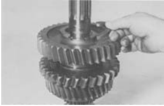
Figure 64 - Position 1st gear split washer in groove of mainshaft. NOTE: If a 1st gear thrust washer is used in place of the split washer, position thrust washer on shaft and proceed with Figure 66.
