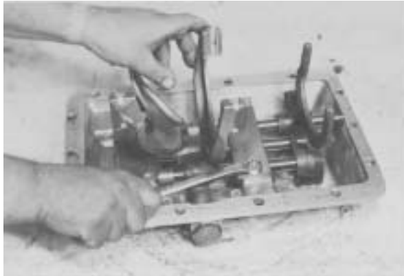
Figure 82 - Remove front and rear rail support cap-screws.
