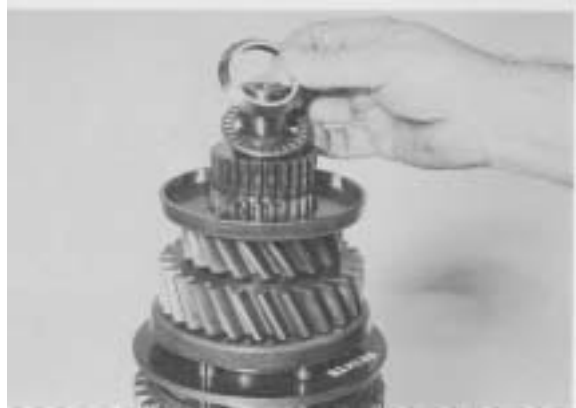
Figure 20 - Remove shift hub thrust bearing and bearing race.
