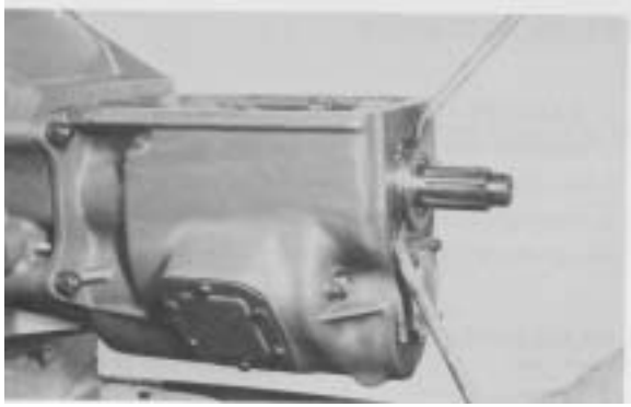
Figure 5 - Tap on main drive gear to move mainshaft to the rear about ¼" [6,35 mm]. Use pry bars as shown to remove rear bearing cup and locating ring.
