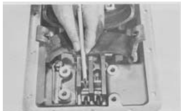
Figure 131 - Note position of tapered interlock pins and shift rails.
