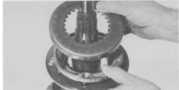
Figure 26 - Remove 3rd gear synchronizer cup and synchronizer assembly. NOTE: There is a variation in the mainshaft 1st gear retention. One version has a split washer and a split washer retainer ring. Using a three-legged puller (as shown in Figure 27), pull against split washer retainer ring to remove rear bearing
