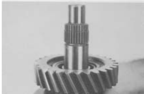
Figure 43 - Using caution as NOT to catch the needle rollers on the edge of a spline or snap ring groove, install 3rd gear on mainshaft.
