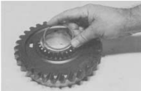
Figure 54 - With clutching teeth of Reverse gear up, coat inside diameter of gear with a high quality heavy grease. This will hold needle rollers in position while assembling. Insert one roller spacer.
