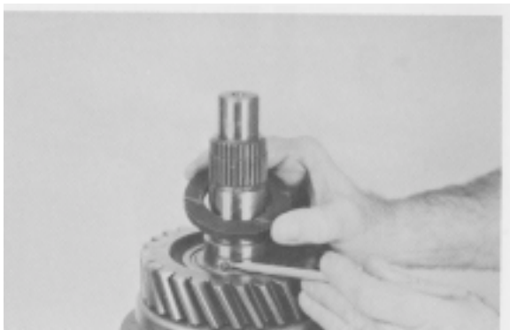
Figure 44 - Install 3rd speed thrust washer lock ball, washer and washer retainer ring.
