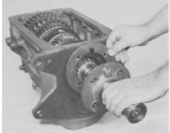
Figure 165 - Using example .035 - .037 --average .036 + .016 = .052 shim pack, position shim pack and main drive gear bearing cap on main drive gear. Lube oil groove in bearing cap MUST be at the top.
