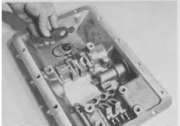
Figure 116 - Remove 1st & Reverse rocker arm.
