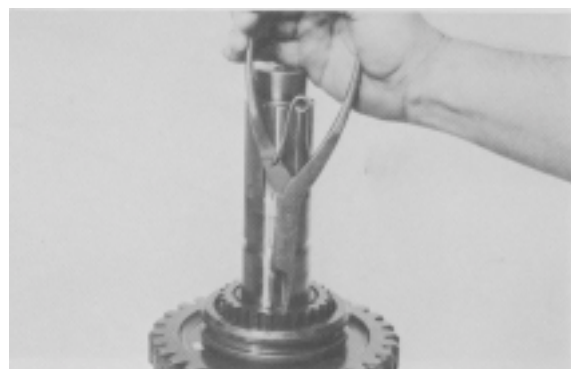
Figure 32 - Remove 1st & Reverse shift hub sleeve retainer ring.
