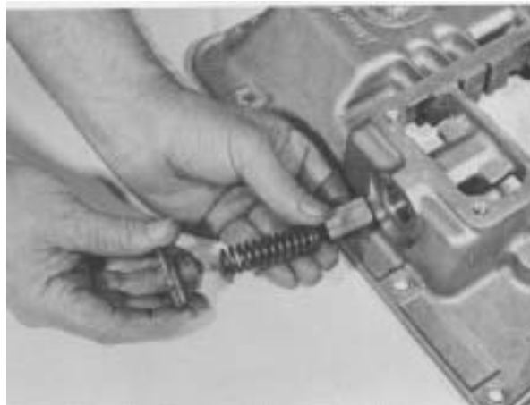
Figure 118 - Remove reverse latch plunger spring and plunger.
