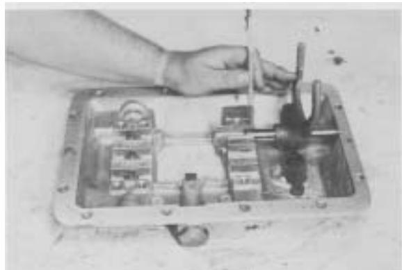
Figure 87 - Using a small magnet, remove the 1st & Reverse shift fork rod lock pin.
