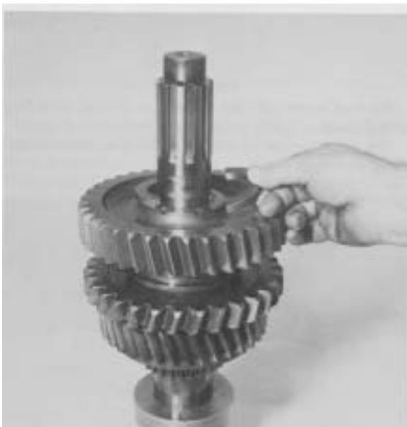
Figure 30 - Remove 1st gear split washer
