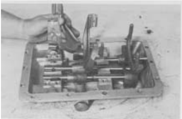
Figure 100 - Position the 4th & 5th shift rail and fork assembly in rail groove over mesh lock ball and spring.
