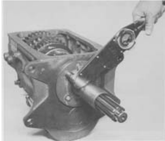
Figure 166 - Install capscrews and tighten 15 - 20 ft.lbs. torque [20,4 - 27,1 N.m.].
