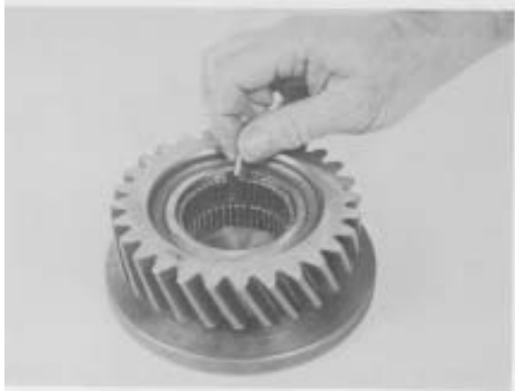
Figure 40 - Lay up second row of needle rollers.
