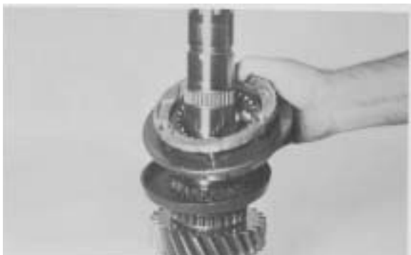
Figure 45 - Turn mainshaft over. Install 3rd gear synchronizer cup and 2nd & 3rd synchronizer assembly.
