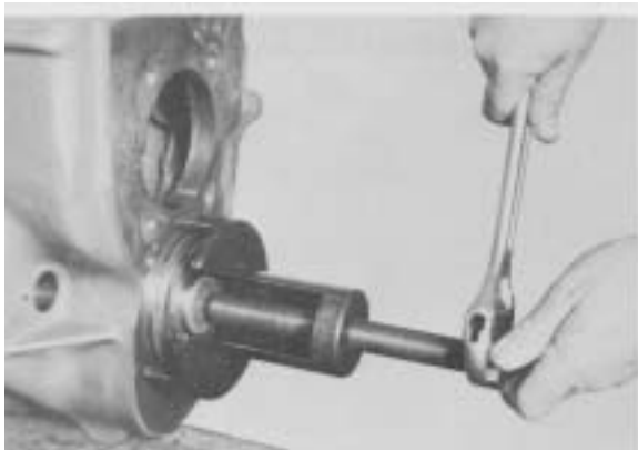
Figure 15 - Pry countershaft to the rear. Using a suitable puller, remove countershaft bearing
