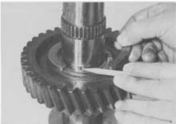
Figure 36 - Remove 2nd gear split washer. CAUTION: Do NOT lose locating ball. This is to prevent split washer from spinning.
