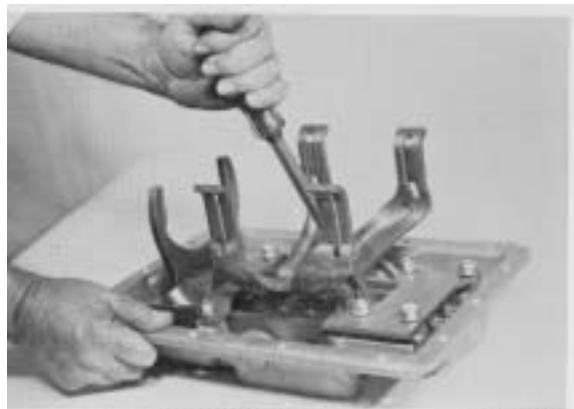
Figure 103 - With control cover in neutral, pry 4th & 5th shift fork to 4th speed position (toward the rear of cover).
