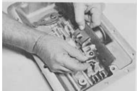
Figure 124 - Align one tapered interlock cross pin with hole in 1st & Reverse shift rail. Position rail on poppet ball with rail in neutral position.
