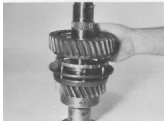
Figure 51 - Using caution as NOT to catch the needle rollers on the edge of a spine or snap ring groove install 2nd gear on mainshaft.
