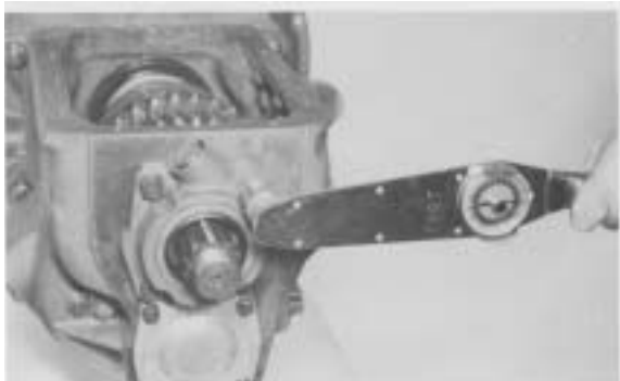
Figure 156 - Install bearing cap bolts. Tighten bolts 35 - 45 ft.lbs. torque [47,5 - 61,0 N.m.].
