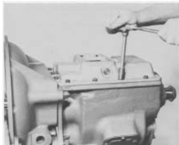
Figure 2- Remove control cover capscrews and control cover.
