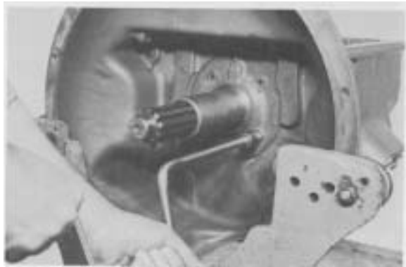
Figure 6 - Remove main drive gear cap bolts.
