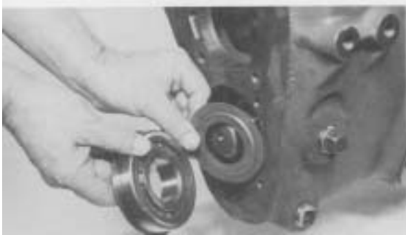
Figure 140 - Position rear bearing oil baffle as shown and start rear bearing.
