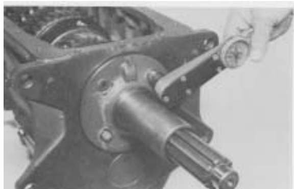
Figure 160 - Install two capscrews 180 Degrees apart and torque screws to 15 inch lbs. [1.7 N.M.].
