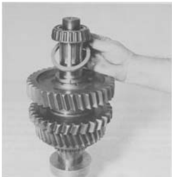
Figure 29 - Remove rear bearing and split washer retainer ring.
