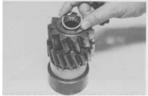
Figure 148 - Position roller spacer on second row of rollers. Grease rollers to hold in place.
