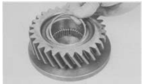
Figure 39 - Position roller spacer on first row of rollers.
