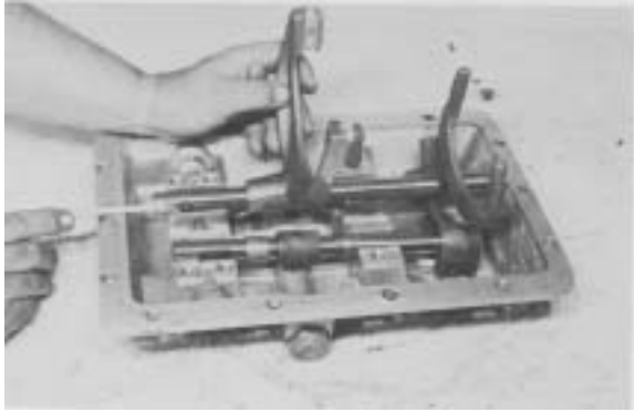
Figure 99 - Install interlock cross pin in 2nd & 3rd shift rail. Position 2nd & 3rd shift rail and fork assembly in rail groove over mesh lock ball and spring. Make certain cross pin is in position in rail. (See Figure 94-A).
