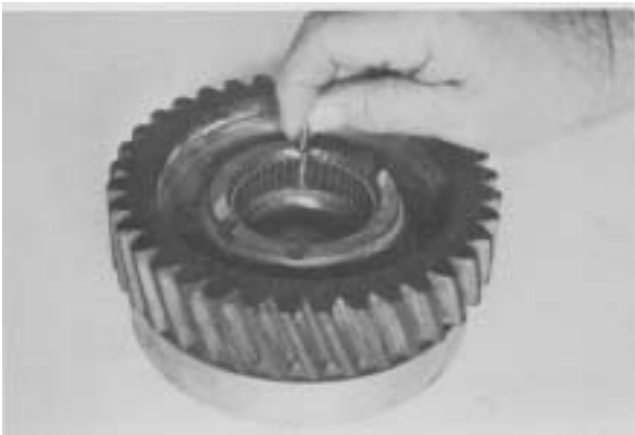
Figure 48 - Lay up second row of needle rollers.
