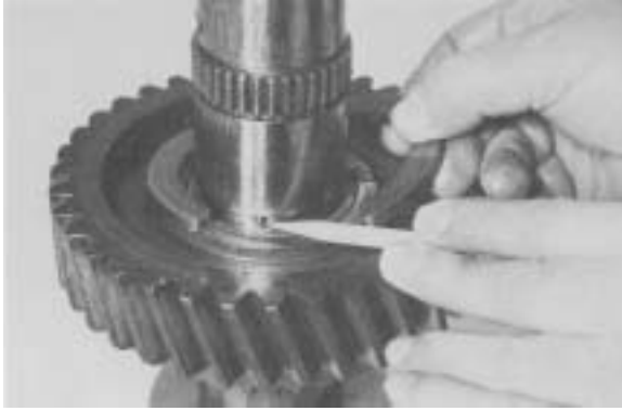
Figure 52 - Position 2nd gear split washer locating ball in shaft. Install split washer in washer groove with ends of washer together at locating ball.
