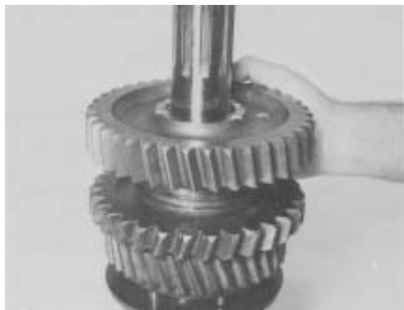
Figure 62 - With clutching teeth of 1st gear down, follow same procedure used in Figures 54 thru Figure 57 to install needle rollers and spacers. Install 1st gear on mainshaft.
