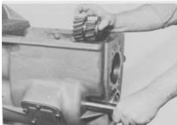
Figure 13 -Remove reverse idler gear and thrust washers. NOTE: Idler gear has loose needle rollers in it. Do NOT lose these rollers.
