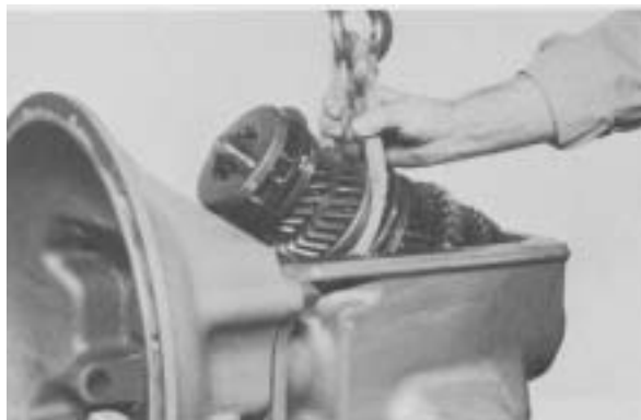
Figure 152 - Install mainshaft assembly into transmission case as shown.
