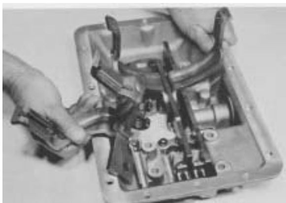
Figure 129 - Position 4th & 5th shift fork and rail on poppet ball in neutral.
