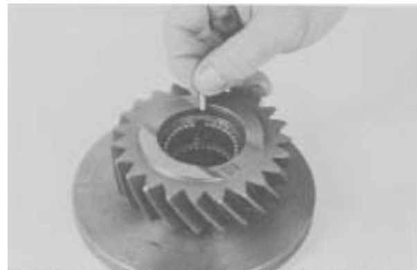
Figure 69 - Lay up second row of needle rollers.
