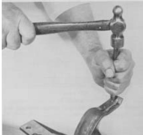
Figure 119 - If fork bushings are worn, secure fork in a vise equipped with soft jaws and remove worn bushings with a drift. Install new bushings in fork. Turn fork over on anvil of vise and secure bushing in fork using a prick punch and upsetting bushing metal on outside of fork.
