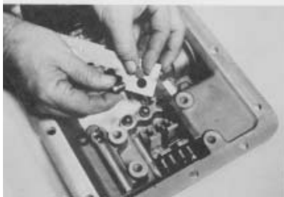
Figure 112 - Use caution as NOT to lose interlock cross pin, interlock tapered pins or mesh lock poppet balls.
