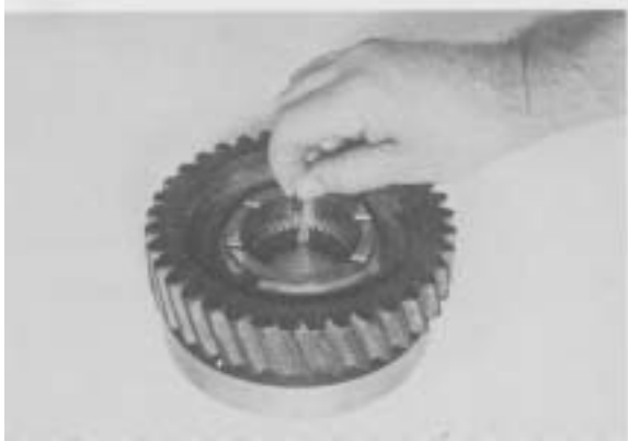
Figure 46 - With clutching teeth of 2nd gear down, coat inside diameter of gear with a high quality heavy grease. This will hold needle rollers in position while assembling. Lay up first row of needle rollers.
