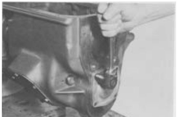
Figure 10 - Remove reverse idler lock and countershaft rear bearing cap bolts.
