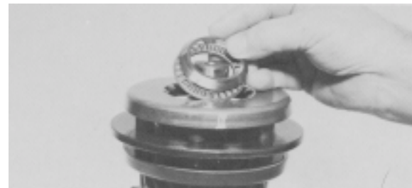
Figure 74 - Grease thrust bearing and install bearing and bearing race on mainshaft.
