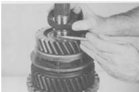
Figure 24 - Remove 3rd gear thrust washer. Use caution as NOT to lose lock ball.
