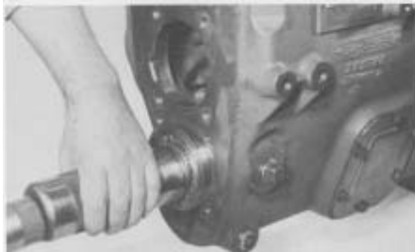
Figure 141 - Drive rear bearing on countershaft and into rear bearing bore. NOTE: Countershaft drive gear must be supported on each side with a 1/4" [6,35mm] flat bar to prevent damage to countershaft pilot bearing.
