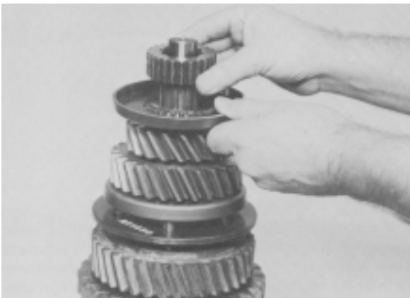
Figure 72 - Position 4th gear synchronizer cup on clutching teeth of 4th gear. NOTE: Chamfer on I.D. of 4th & 5th shift hub sleeve must go down. Install shift hub sleeve on shaft.
