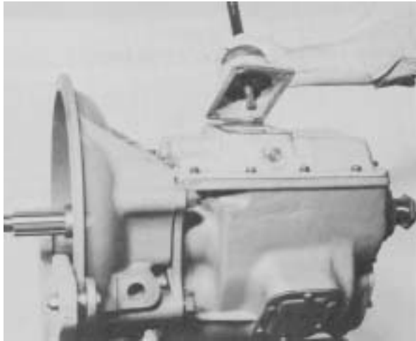
Figure 1- Remove shift lever control top or remote control assembly.
