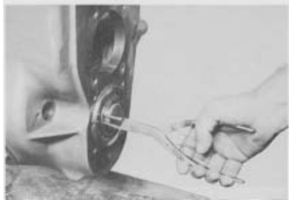
Figure 14 - Remove countershaft rear bearing retainer ring.
