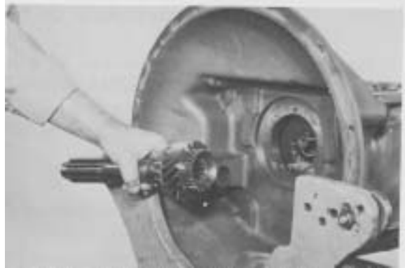
Figure 8 - Remove main drive gear and bearing assembly.
