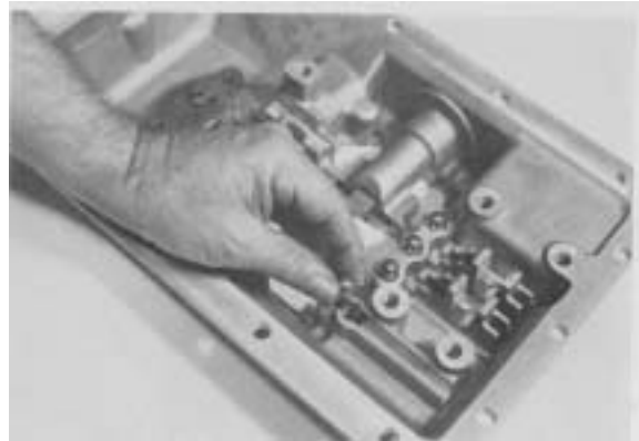
Figure 114 - Remove mesh lock poppet balls, quantity 4.
