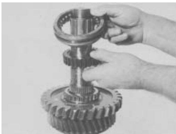
Figure 60 - Position 1st and Reverse shift hub sleeve and hub on mainshaft. NOTE: Counterbore in shift hub sleeve must be up.
