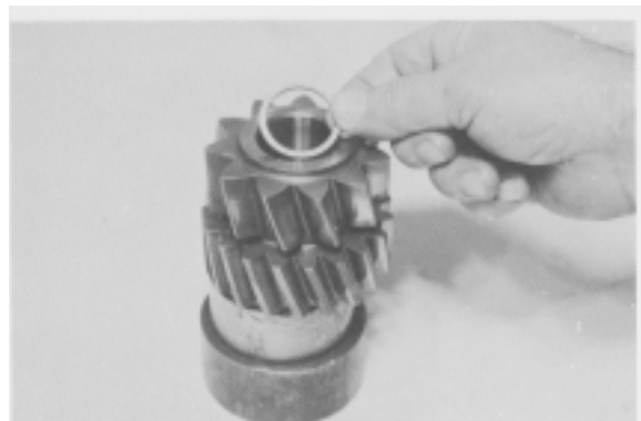
Figure 144 - Coat inside diameter of reverse idler gear with high quality heavy grease. This will hold needle rollers in position while assembling. Insert one roller spacer.
