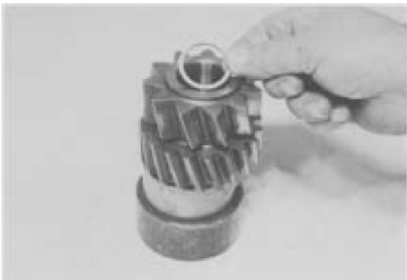
Figure 146 - Position roller spacer on first row of rollers.
