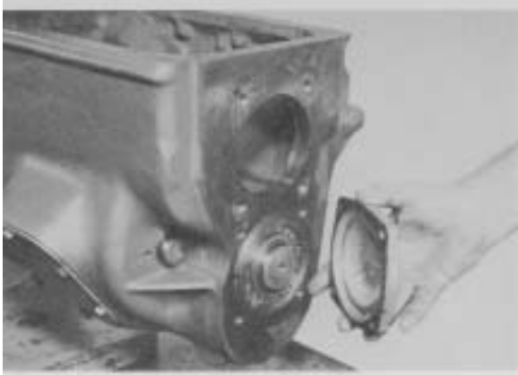
Figure 11 - Remove countershaft rear bearing cap.
