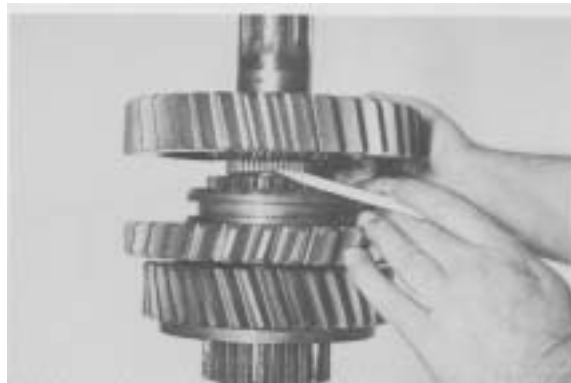
Figure 31 - Remove 1st gear. Use caution as NOT to lose needle rollers under 1st gear. 1st gear was removed in Figure 28 for thrust washer retention. Further disassembly of the mainshaft will be identical in both versions.
