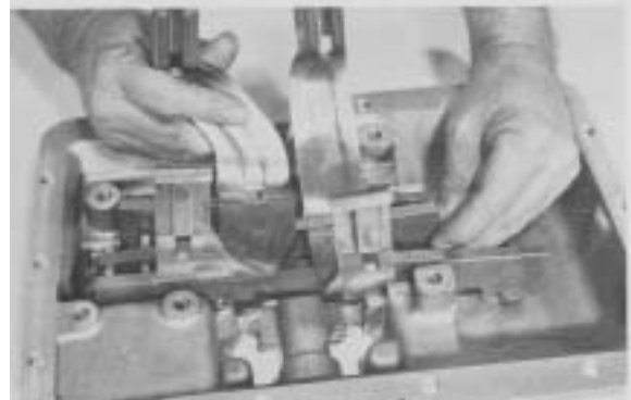
Figure 130 - Slightly raise rear of 4th & 5th shift rail and align 2nd interlock tapered pin with cross hole in 4th & 5th shift rail.
