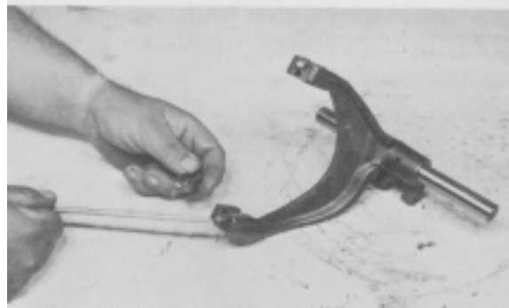
Figure 91 - If the 2nd, 3rd, 4th or 5th shift fork bushing is to be replaced, remove worn bushings from fork. Install new bushing and bend bushing tab over top and bottom of fork.
