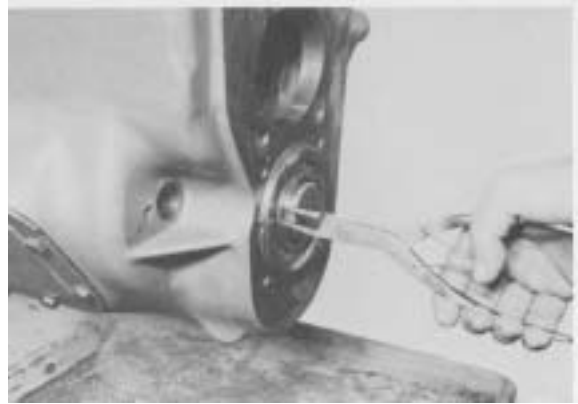
Figure 142 - Install countershaft rear bearing retainer ring.
