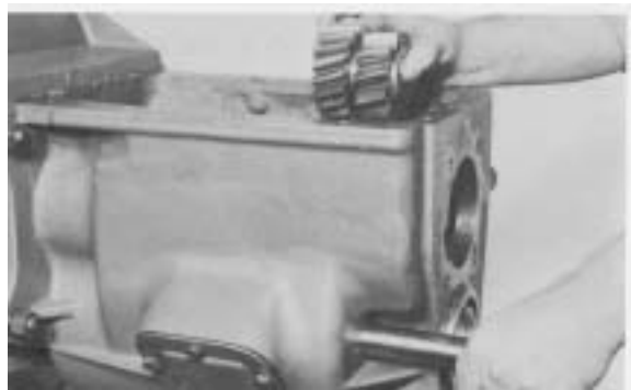
Figure 150 - Carefully position reverse idler gear in housing. Use caution as NOT to disrupt needle rollers. Insert idler shaft through case and idler gear needle rollers. NOTE: Idler shaft lock groove MUST line up with lock screw hole. Drive shaft into position. Install shaft lock and capscrew.
