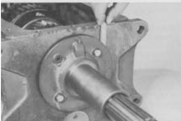
Figure 163 - Using a taper gauge at a capscrew, as shown, record gap between bearing cap and housing. Example: .035 [0,88mm].
