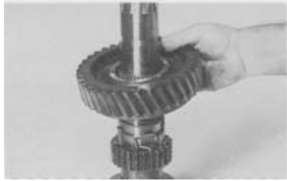
Figure 37 - Remove 2nd gear. Use caution as NOT to lose needle rollers under 2nd gear.
