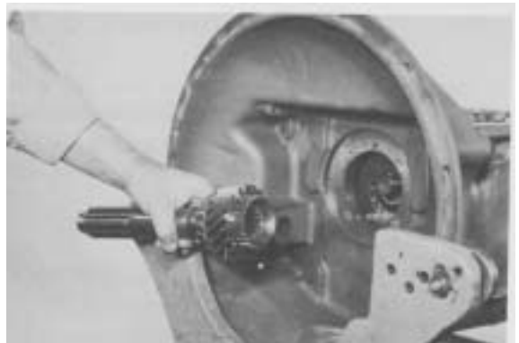
Figure 9 - Using a hoist (if available) and a heavy rope, lift mainshaft assembly from transmission case. Mainshaft can be removed by hand, but is quite difficult to handle.
