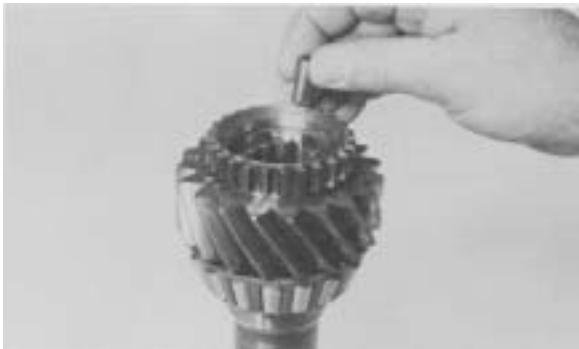
Figure 78 - Press new taper bearing on drive gear. Turn gear over. Using a high quality heavy grease, coat roller bearing surface. Place rollers in grease as shown.
