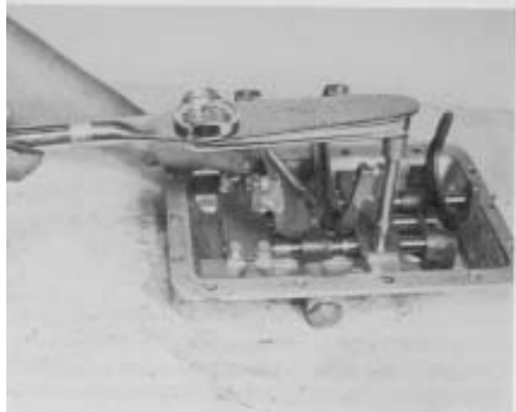
Figure 102 - Tighten support capscrews 20 - 25 ft.lbs. torque [27,2 - 33,8 N.m].
