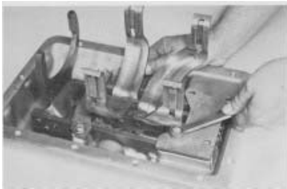
Figure 104 - Remove front rail support cap screws.
