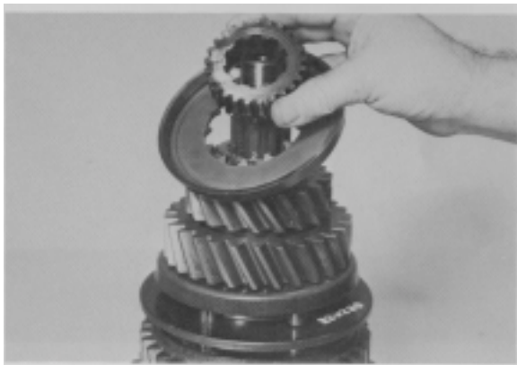
Figure 21 - Remove 4th & 5th shift hub sleeve and 4th speed synchronizer cup.
