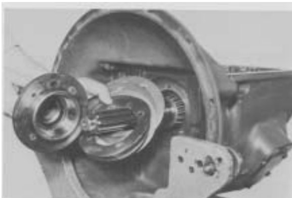
Figure 7 - Using a soft hammer, tap on threaded end of mainshaft. Move mainshaft toward main drive gear. From front of transmission, remove main drive gear bearing cap and shims.
