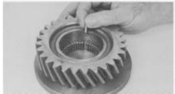
Figure 38 - With clutching teeth of 3rd gear down, coat inside diameter of gear with a high quality heavy grease. This will hold needle rollers in position while assembling. Lay up first row of needle rollers.
