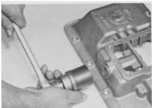
Figure 117 - Remove reverse latch plunger spring retaining plug.
