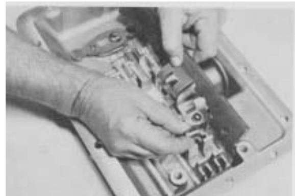
Figure 125 - Note position of tapered interlock cross pin in relation to rail.
