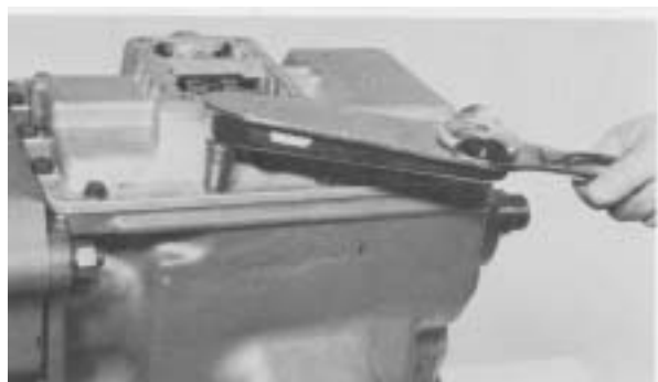
Figure 168 - When installing control assembly, install and tighten center rear screw first, center front screw second and then remaining screws. Tighten screws 20 - 25 ft. lbs. torque [27,1 - 33,8 N.m].
