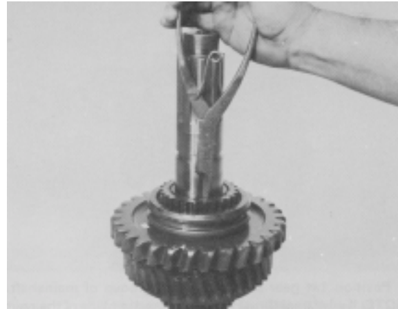
Figure 61 - Install shift hub sleeve retainer ring.
