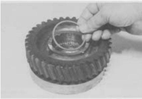
Figure 47 - Position roller spacer on first row of rollers.
