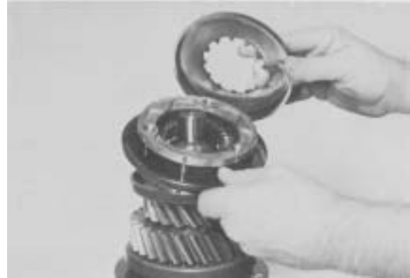
Figure 73 - Install 4th & 5th synchronizer assembly and 5th speed synchronizer cup on shaft.
