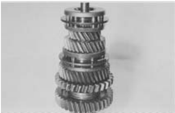
Figure 18 - Position mainshaft in a suitable stand. A vise may be used if soft jaws are utilized.
