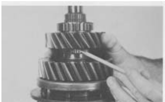
Figure 22 - Remove 4th speed gear. Use caution as NOT to lose needle rollers under gear.
