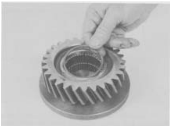
Figure 41 - Position outer roller spacer on second row of rollers. Grease rollers to hold in place.
