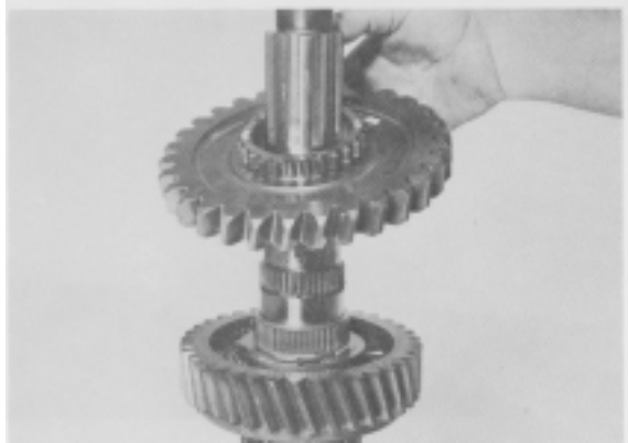
Figure 34 - Remove reverse gear. Use caution as NOT to lose needle rollers under reverse gear.
