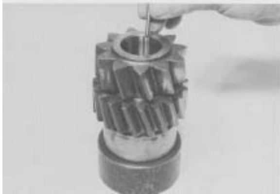
Figure 145 - Lay up first row of needle rollers in spacer.
