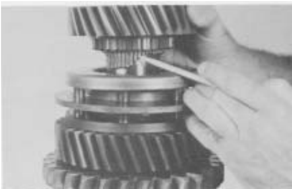
Figure 25 - Remove 3rd speed gear. Use caution as NOT to lose needle rollers under gear.
