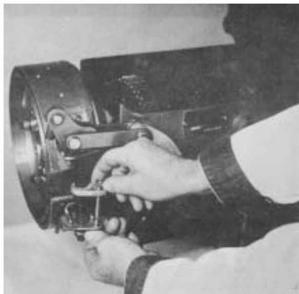
Figure 6 -Remove jam nuts and brake band locating screw.
