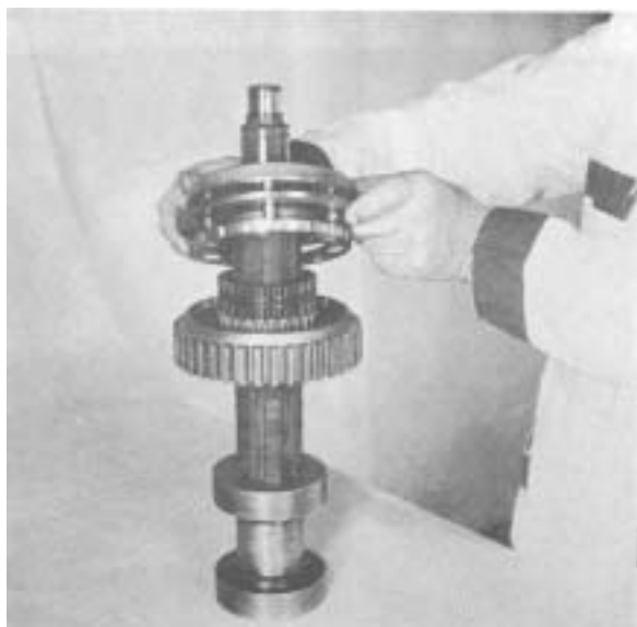
Figure 54 - Install 2nd & 3rd synchronizer assembly.
