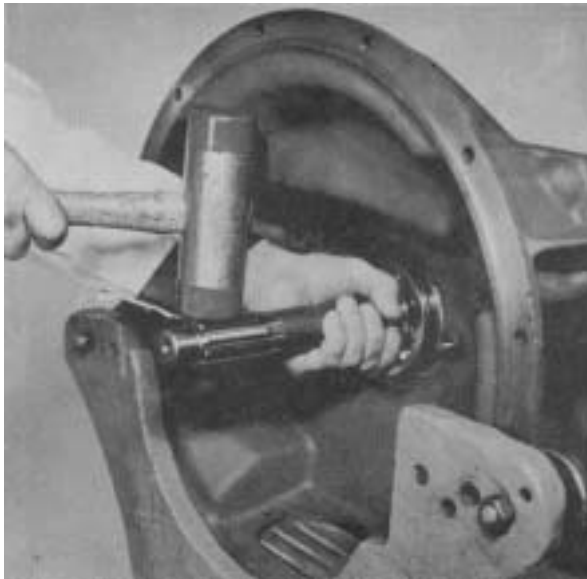
Figure 16 -Remove main drive gear. Use caution as not to drop mainshaft spigot bearing rollers in transmission case.
