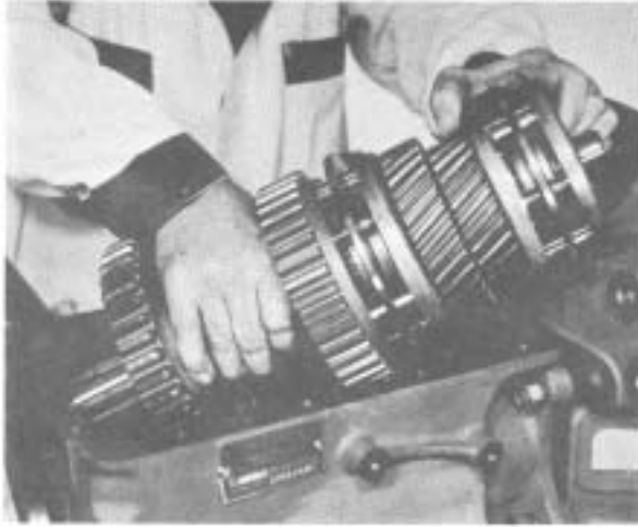
Figure 69 - Install mainshaft assembly into transmission case as shown.
