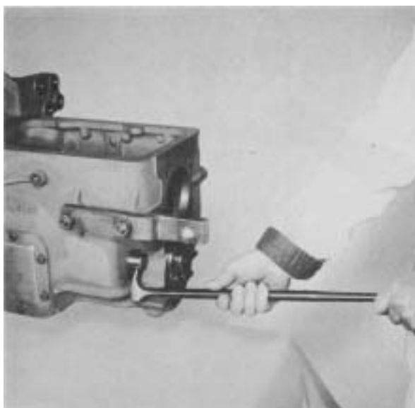
Figure 19 -Remove reverse idler shaft lockscrew and lock. Using a suitable puller remove reverse idler shaft.
