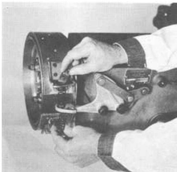
Figure 80 - Install brake release springs and cam lever shoe as shown.
