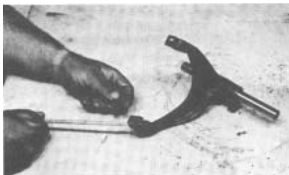
Figure 12 - Install reverse latch plunger, spring, pin and plunger spring plug.
