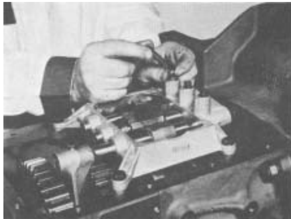
Figure 84 - With transmission shifted into neutral, install shift control assembly. 2nd & 3rd and 4th & 5th shift forks set over shift hubs, 1st & reverse fork enters slot on 1st & reverse gear. Tighten bolts 20 to 25 ft. lbs. torque [27,2 - 33,8 N.m]. Position three mesh lock balls and springs in support housing.
