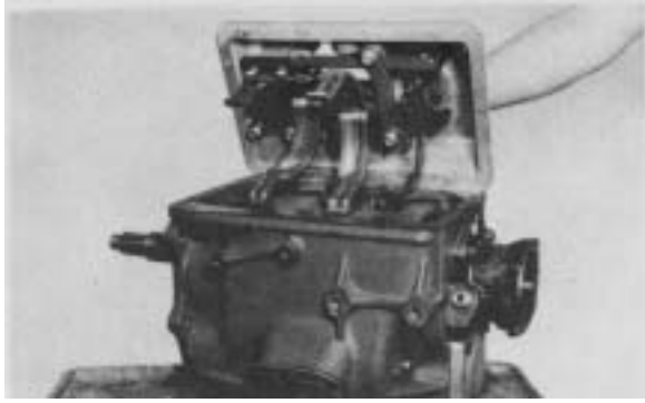
Figure 71 - With new gasket in position and with transmission in neutral, position control cover over gears aligning shift forks in shift cover with gear shift hubs. If control cover is in neutral and transmission is in neutral, transmission drive gear should turn without output shaft turning.
