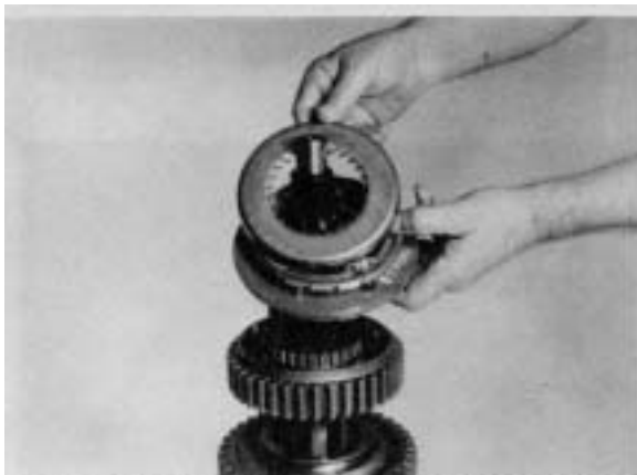
Figure 102 - Install 2nd & 3rd synchronizer and synchronizer cup on shift hub sleeve.
