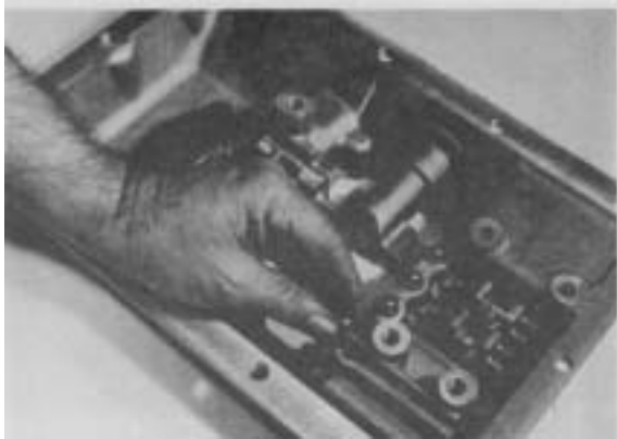
Figure 47 - Remove mesh lock poppet balls, quantity 4.
