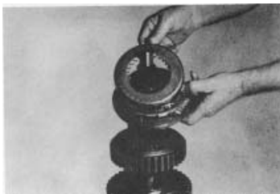
Figure 27 - Remove 2nd & 3rd synchronizer cup and synchronizer assembly.
