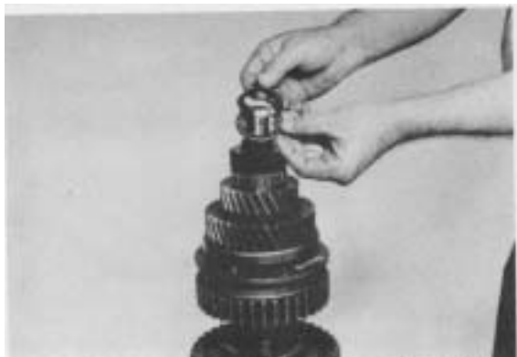
Figure 23 - Remove shift hub bearing race and bearing.
