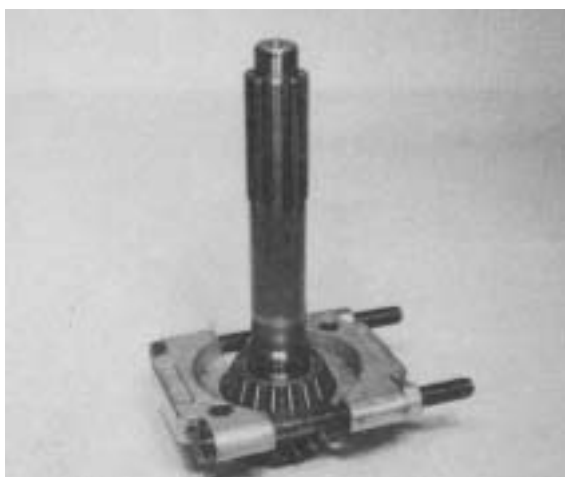
Figure 34 - If main drive gear taper bearing is to be removed, split puller shown is recommended.
