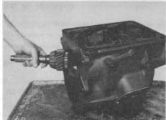
Figure 8 - Remove main drive gear and bearing assembly.
