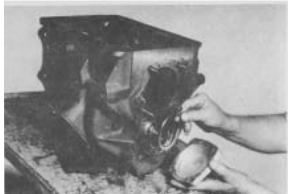
Figure 14 - Remove countershaft rear bearing cap and bearing spacer ring.
