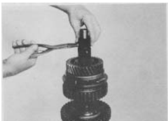
Figure 25 - Remove 3rd gear retaining ring.
