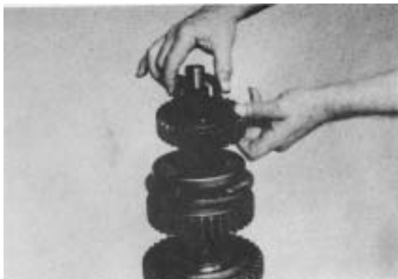
Figure 26 - Remove locating washer and 3rd gear.
