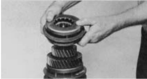
Figure 107 - Install the 4th & 5th speed synchronizer and synchronizer cups on shift hub sleeve.
