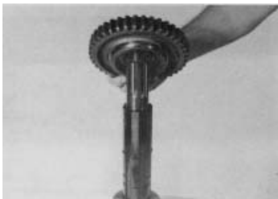
Figure 33 - Remove 1st & Reverse sliding gear.
