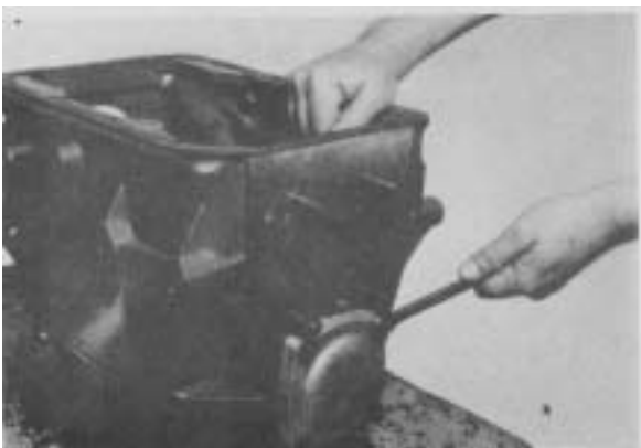
Figure 13 - Remove countershaft rear bearing cap bolts & washers.
