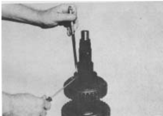
Figure 28 - Remove 2nd & 3rd shift hub sleeve retainer ring.
