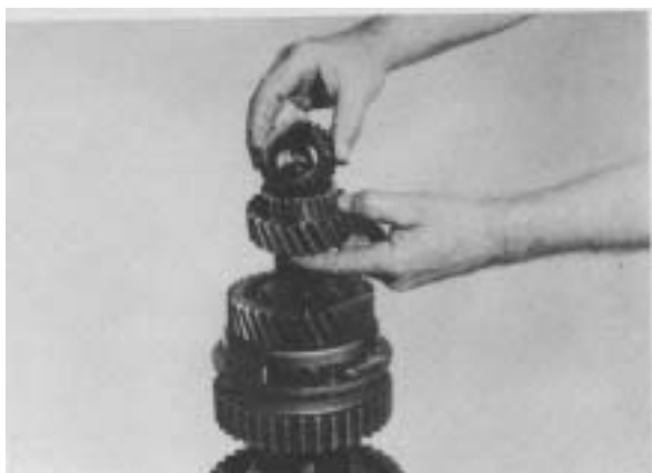
Figure 24 - Remove shift hub sleeve and 4th gear.
