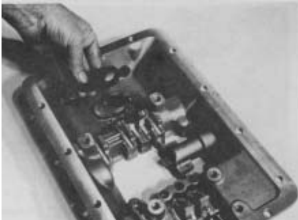
Figure 54 - Position 1st & Reverse rocker arm on pivot pin as shown.
