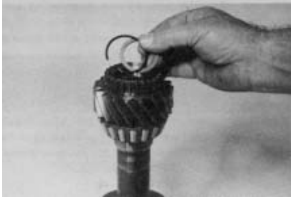
Figure 95 - Install roller bearing washer and retainer ring.
