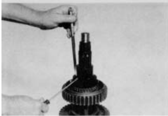
Figure 101 - Install shift hub sleeve retainer ring
