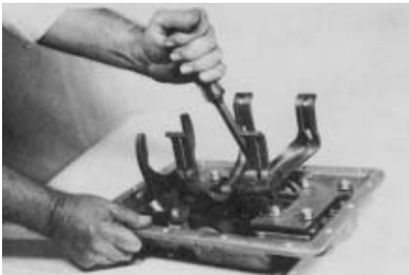
Figure 31 - Remove front rail support cap screws.
