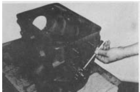
Figure 14 - Remove countershaft rear bearing cap and bearing spacer ring.
