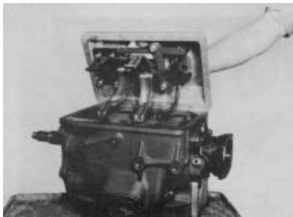
Figure 2 - Remove control cover assembly from transmission.
