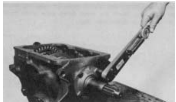
Figure 133 - Install capscrews and tighten 15 to 20 lb. ft. torque [20,4 - 27,1 N,m].
