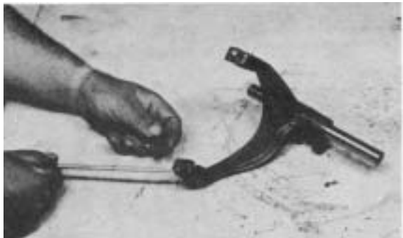
Figure 82 - Remove mesh lock spring and lock ball, 3 each. Remove crossover interlock balls, 4 each.
