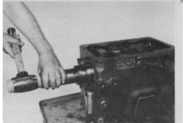
Figure 122 - Install mainshaft rear bearing cup
