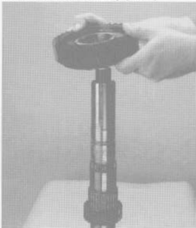
27. Remove 2nd speed gear.
