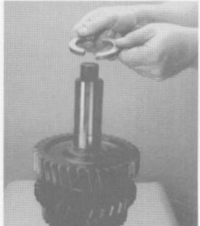
17. Remove the 1st gear split washer.
