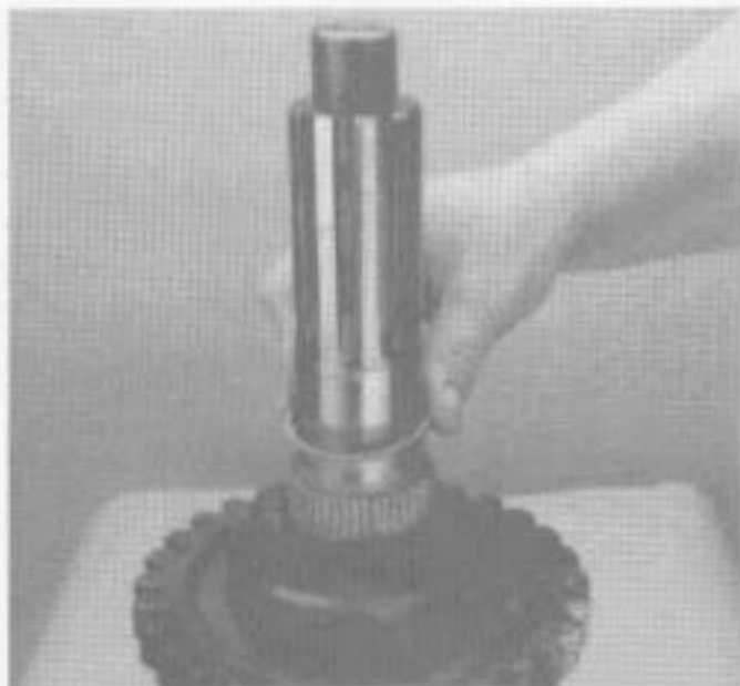
10. Coat the mainshaft 1st gear position with a high quality grease. Lay a row of needle bearings around the mainshaft, 44 needle bearings. Place a spacer ring over the top of the bearings. Lay a second row of 44 needle bearings around the mainshaft on top of the spacer ring. Install a spacer ring over the top of the second row of needle bearings.
