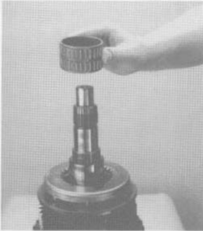
17. Install mainshaft 3rd speed gear bearing.
