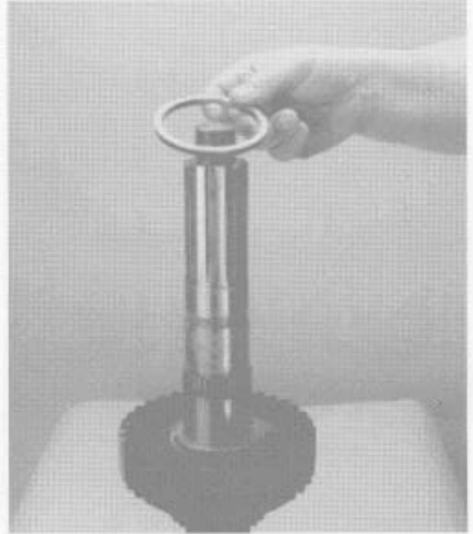
25. Remove 2nd gear split washer retainer ring.
