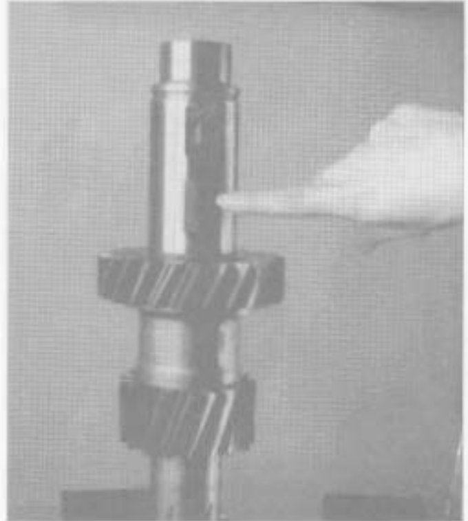
13. Remove 4th gear key from the countershaft
