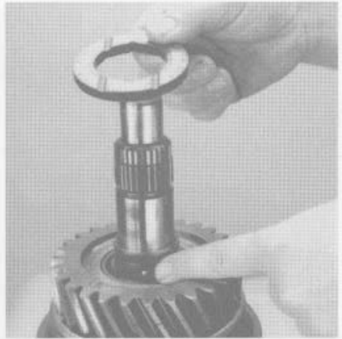
10. Remove 3rd speed gear thrust washer. Remove the locating ball.
