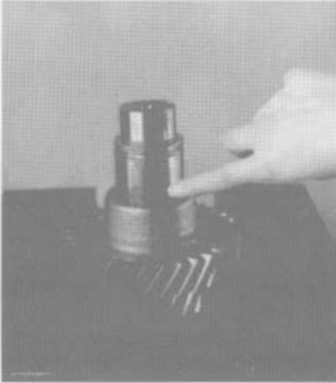
11. Remove the 5th gear key from the countershaft.
