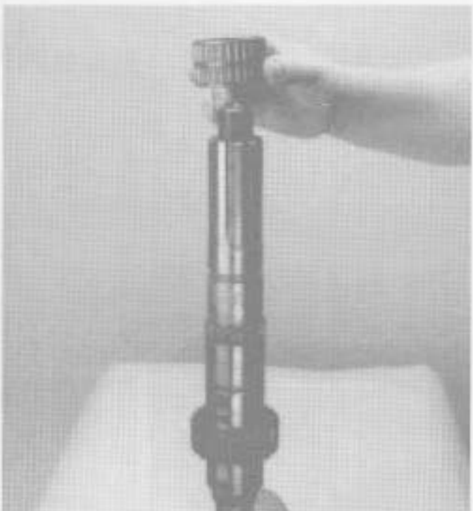
28. Remove 2nd gear bearing.
