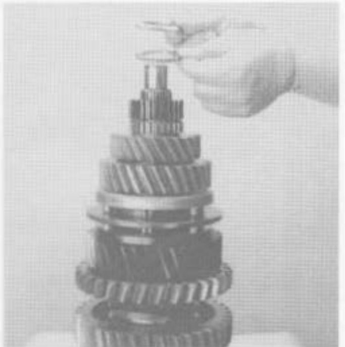
24. Install thrust bearing and bearing race on the mainshaft 4th-5th clutch hub.
