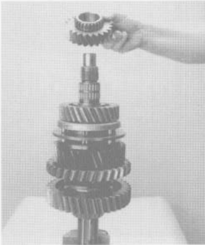
7. Remove the 4th speed gear.
