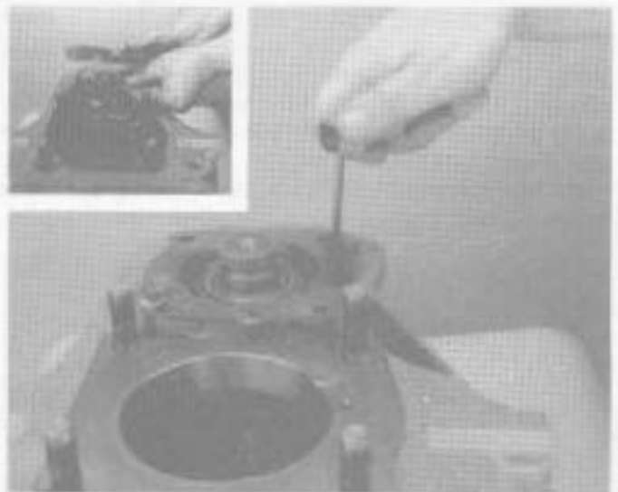
12. Temporarily install new shims into the bearing retainer (inset). Install the retainer and tighten the set screws to the recommended torque.
