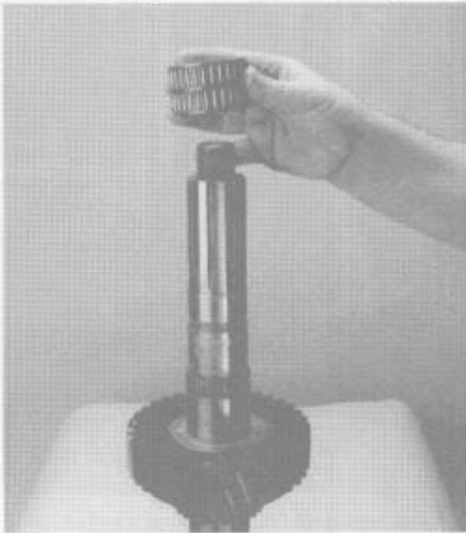
5. Install mainshaft reverse gear bearing.
