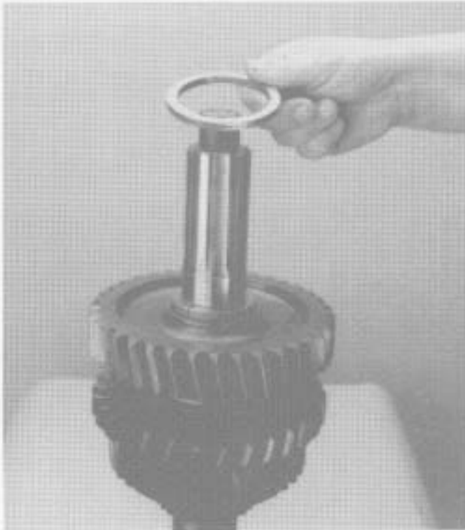
13. Install the split washer retainer ring over the split rings.
