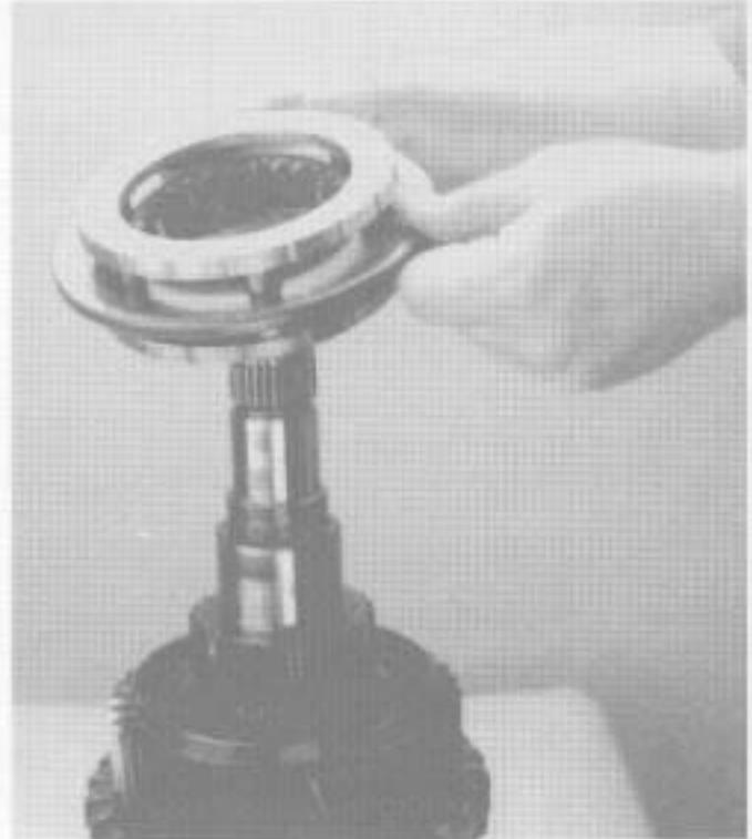
15. Reposition mainshaft in vise so front is up. Install the mainshaft 3rd speed gear synchronizer assembly.
