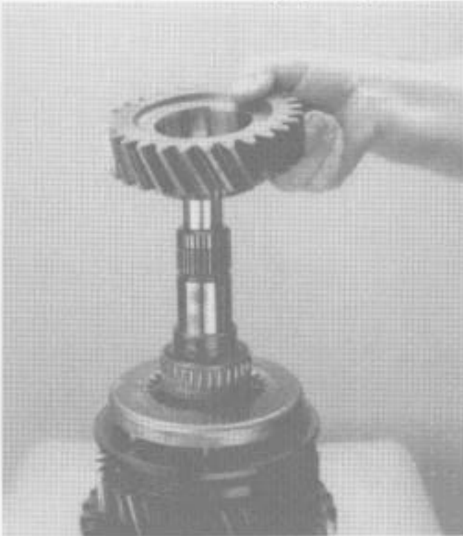
11. Remove the 3rd speed gear.
