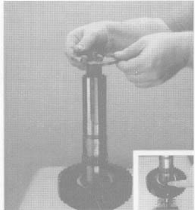
26. Remove the 2nd gear split washer and locating ball (inset).
