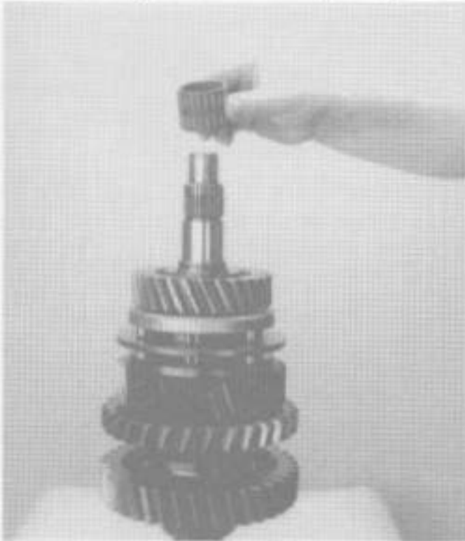
21. Install mainshaft 4th gear bearing.
