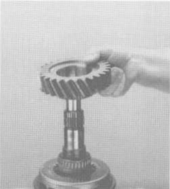
18. Install mainshaft 3rd speed gear, clutching teeth facing down.
