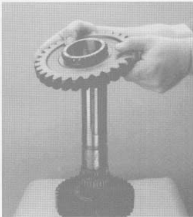
6. Install mainshaft reverse gear.
