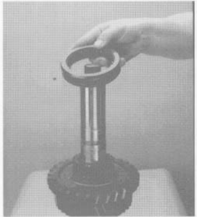
8. Install 1st-reverse gear sliding clutch.
