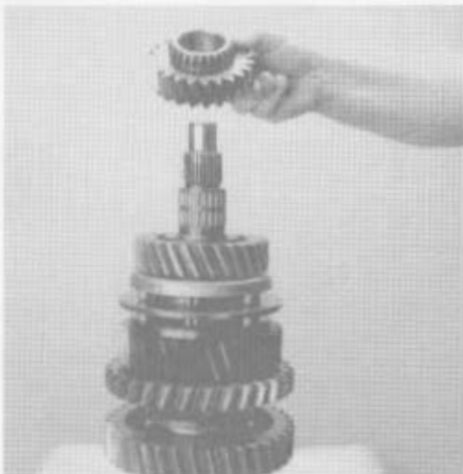
22. Install mainshaft 4th speed gear, clutching teeth facing up.
