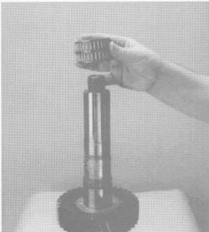
24. Remove the reverse gear bearing.
