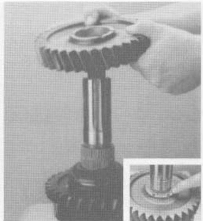
18. Remove the 1st gear. Use caution so not to lose bearing rollers under the 1st gear (inset).
