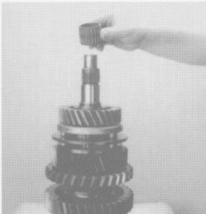
8. Remove 4th gear bearing.
