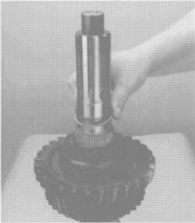
19. Remove the bearing rollers and spacers.
