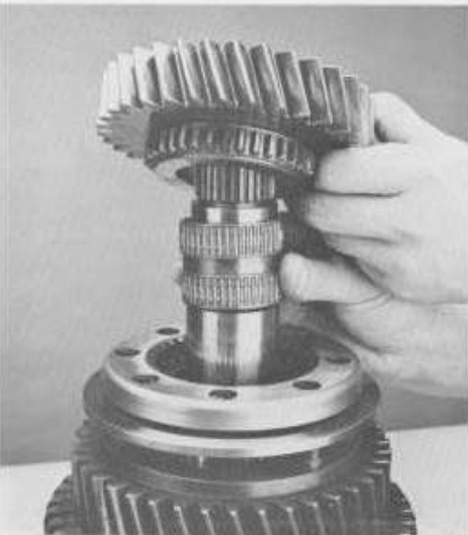
9. Remove 3rd gear, bearings and spacer from main shaft.
