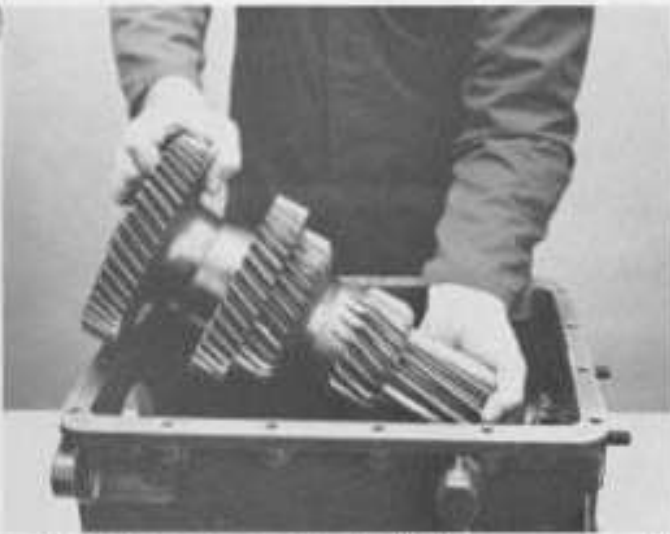
9. Carefully lower countershaft into case.
