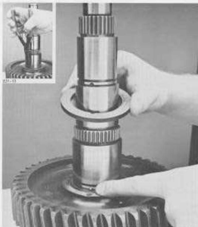
13. Remove snap ring (inset), thrust washer, and locating ball.
