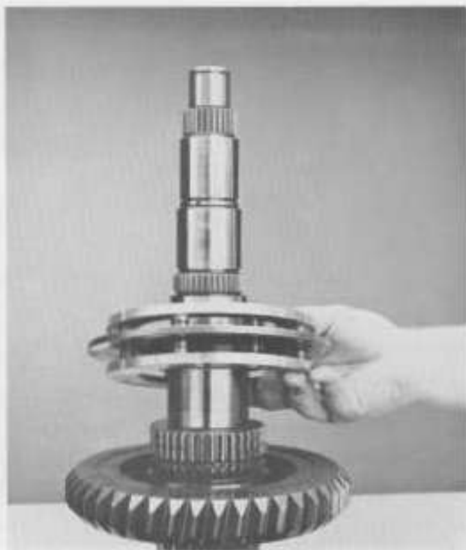
15. Remove 1st speed synchronizer.
