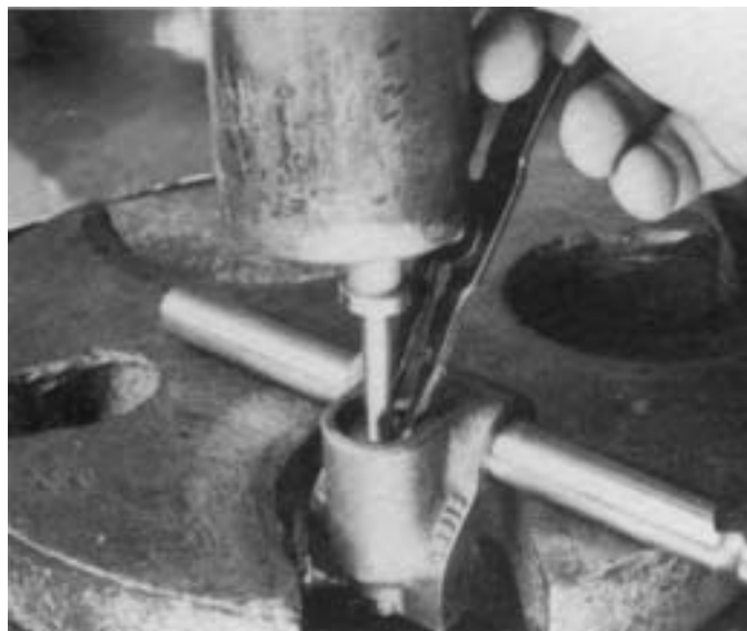
11. Place the shift yoke in a hand press. Depress retaining washer and spring and install the snap ring.
