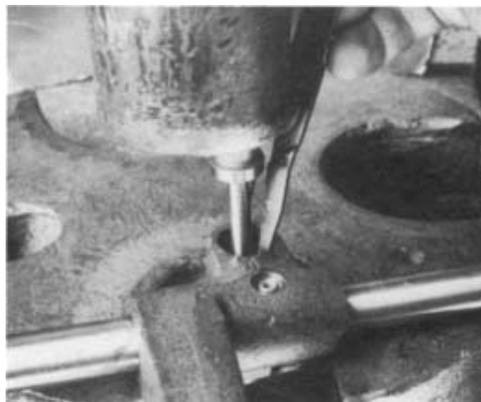
6. Place shift yoke in hand press. Depress retaining washer and spring and install the snap ring.
