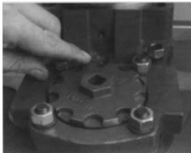
13. Lock transmission in two gears, install the output flange nut and tighten to the specified torque.
