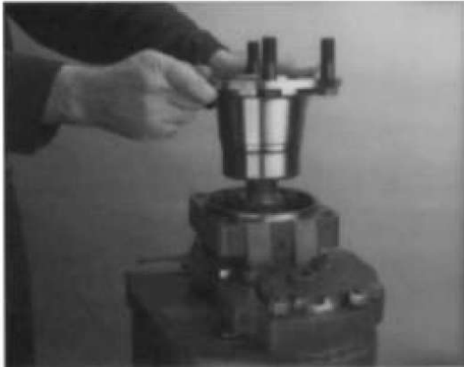
12. Install the output flange on the output shaft.
