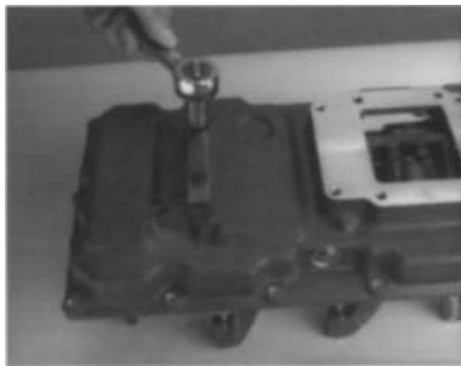
18. Tighten the two detent spring cover cap screws to recommended torque.
