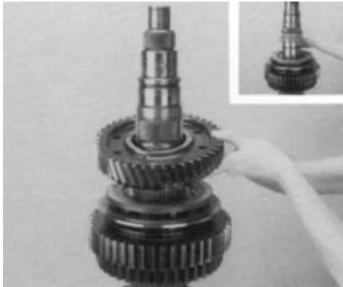
13. Remove 2nd speed gear and 2nd speed gear bearings from the mainshaft (inset).
