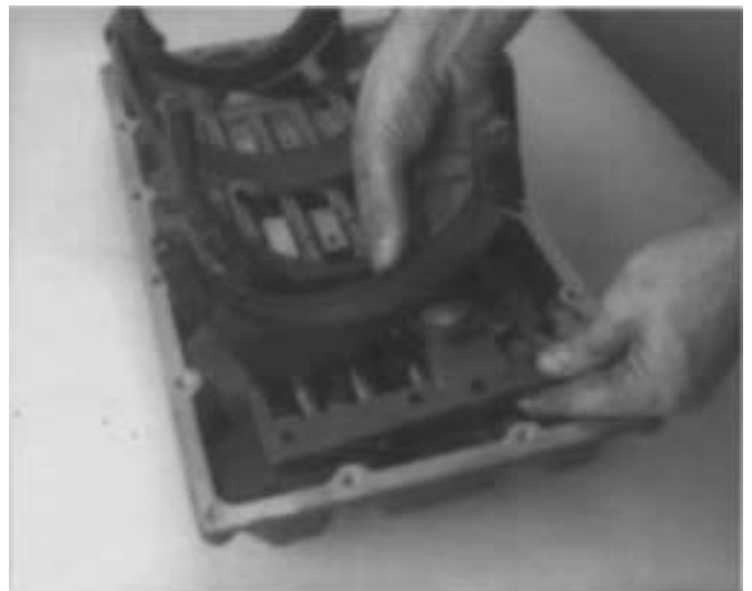
5. Remove fifth-sixth actuator from the shift bar housing.
