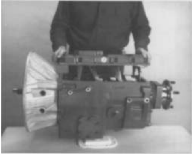
1. Remove capscrews and lift shift bar housing from case.
