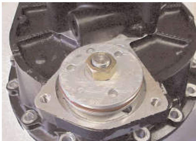
29. Change the 'O' rings in the piston if necessary. Apply silicon lubricant to the 'O' rings and fit the piston, flat face uppermost. Fit the nut.
