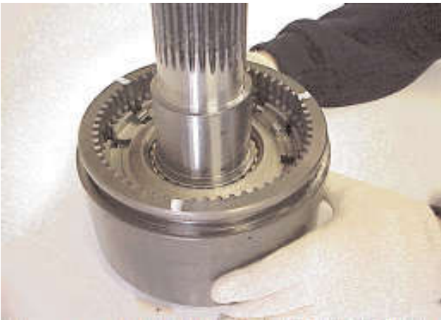
8. Put identifying marks on the synchroniser sliding sleeve in line with the synchroniser plungers, if not already marked, and remove the sleeve and annulus assembly. Note the position of the spring plungers and rollers and remove them from the hub.
