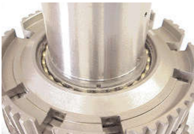
10. Install the retaining snap ring.
