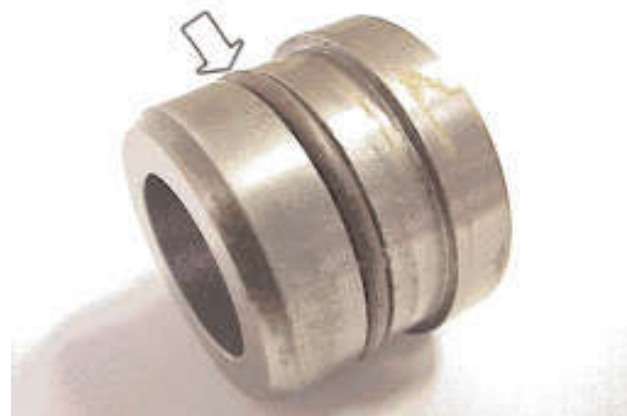
11. Install a new O-ring into the groove on the outer periphery of the bush carrier. Lubricate sparingly with silicone grease
