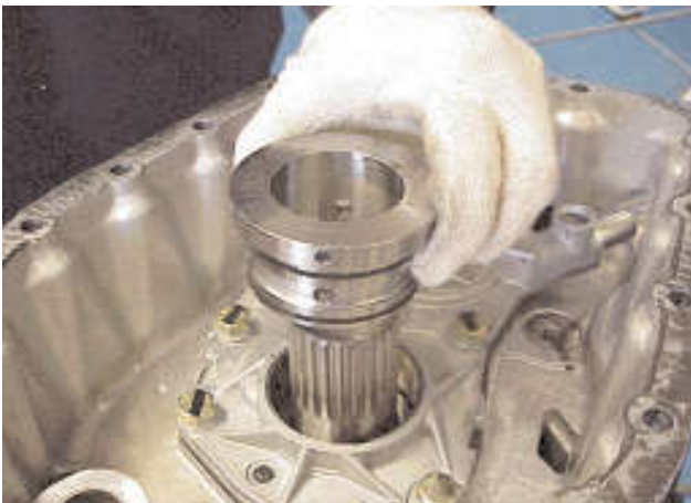
14. Lift out the muff ring taking care not to damage the two sealing rings.
