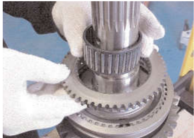
6. Remove the reverse gear needle roller bearing. Lift off the reverse gear flange from the synchroniser hub. Note: There is no synchroniser ring for the reverse gear.
