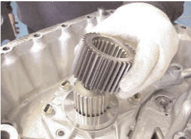
13. Lift off the sun gear.
