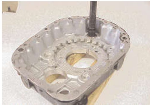
10. Range change selector rod bush - rear case. Drift out the rear bush complete with carrier from the rear case.
