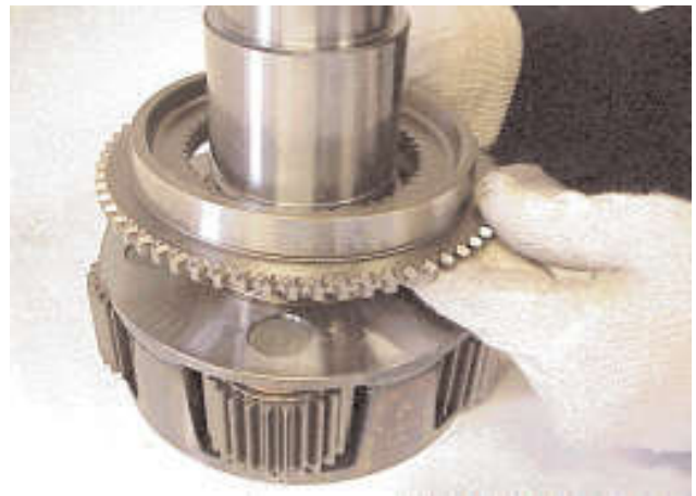
12. Remove the synchroniser flange.
