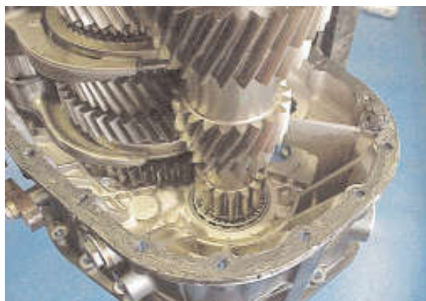
15. Apply sealer to the case mating flange ensuring that there is a continuous bead around the flange and the retaining capscrew holes.
