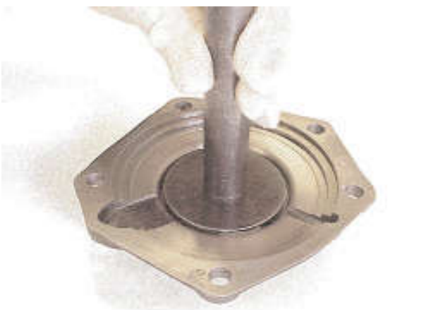
13. If removed, install a new oil seal into the input shaft bearing front cover using the special tool. Press the seal firmly down to the shoulder ensuring the seal is not damaged.
