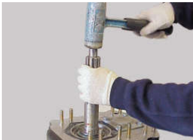
43. Use a soft faced mallet to drive the shaft through the case taking care not to allow the shaft to fall and become damaged.
