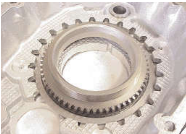
17. Place the synchroniser flange and snap ring onto the spacer ring. On some multi-purpose specification transmissions an additional oil seal should be fitted in the rear case. This should not block off the oil feed hole in the output shaft.
