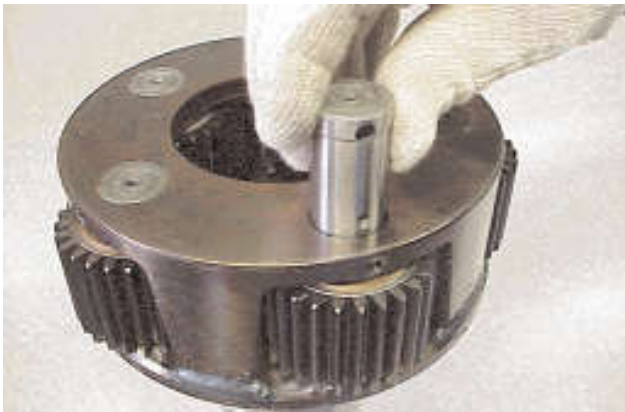
7. Slide in the gear assembly until the bore of the planet carrier and gear assembly align.
