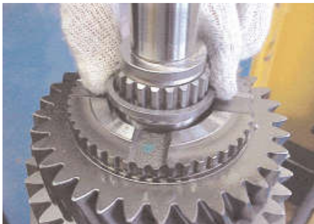
26. Place the 3rd gear bearing spacer ring into the gear against the bearing.
