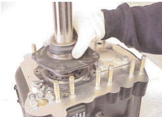
40. Remove the capscrews securing the input shaft cover to the front case half. Remove the cover.
