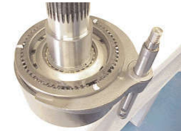
20. Locate the selector fork and shaft assembly into the synchroniser sleeve, threaded end of shaft uppermost.
