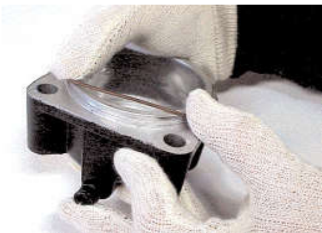
30. Change the 'O' ring if necessary. Apply silicone lubricant to the 'O' ring and to the bore of the cylinder cover.
