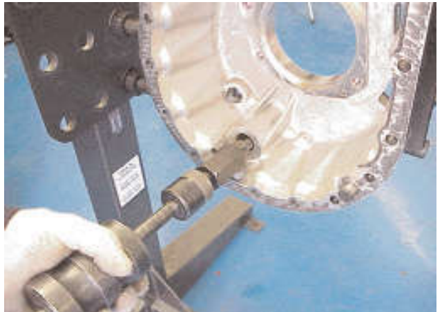
50. Range change selector rod bush - intermediate case. Remove the bush toward the rear using an internal type extractor.
