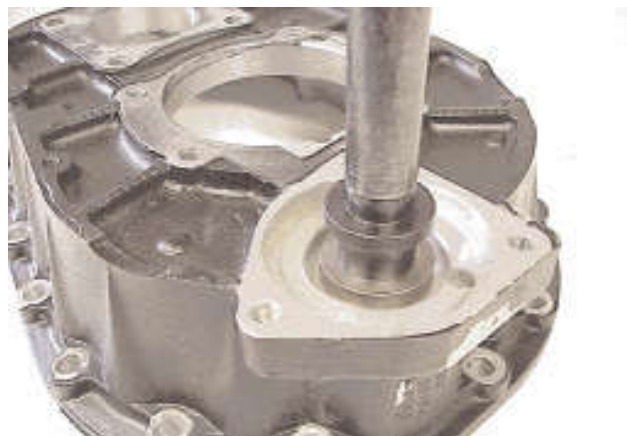
12. Install the bush carrier until the O-ring has just entered the case. Wipe off any surplus grease and apply sealer (Loctite 641) around the exposed part of the bush carrier and drive it into the case using tool E 109-5.
