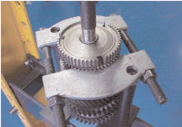
3. Assemble the puller plates over the 3rd/4th gear synchroniser hub and the 3rd gear synchroniser ring and press off the hub, cone and ring, taking care not to damage the synchro ring teeth.
