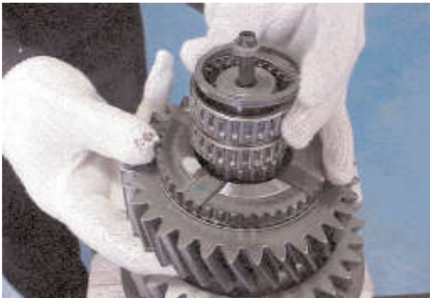
4. Lift off the third gear and 3rd gear needle roller bearing and spacer ring. Note the position of the spacer ring for reassembly.
