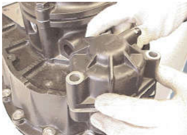
31. Apply a coating of Loctite 5900 to the face of the cylinder cover. Fit the cylinder cover.
