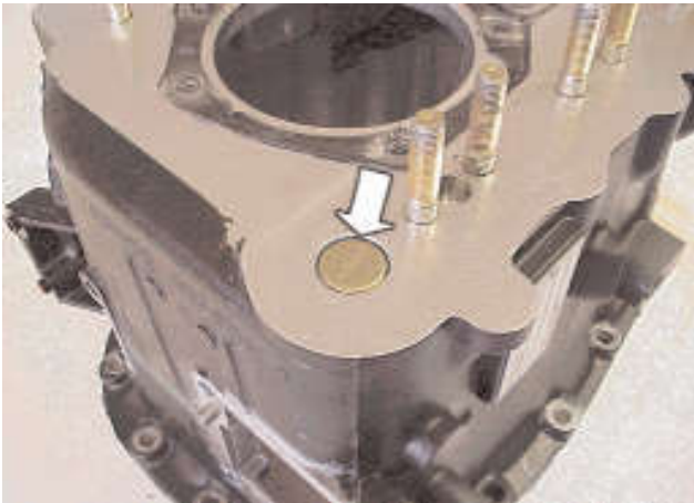
46. If the selector shaft bushes are to be replaced drive the core plug from the front case using a suitable tool. Note; Drive the core plug from inside of the front case.
