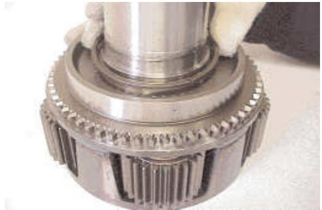
11. Remove the snap ring securing the synchroniser flange to the planet carrier.
