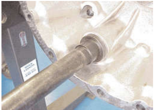
51. Install the new bush until flush with the face of the case bore using tool E 109-5. The bush is prefinished to the correct size. Remove any burrs from the edge of the bush using a fine file or slip stone and check the fit of the selector rod in the bore.
