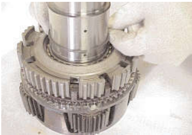
9. Remove the snap ring securing the synchroniser hub bearing to the output shaft.
