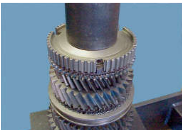
28. Take the heated 3rd/4th synchroniser hub and place it, boss side downwards on the shaft. Ensure that the slots in the hub align with the shoulders on the synchroniser ring. Press the hub fully home and hold under pressure for 3 to 5 minutes.
