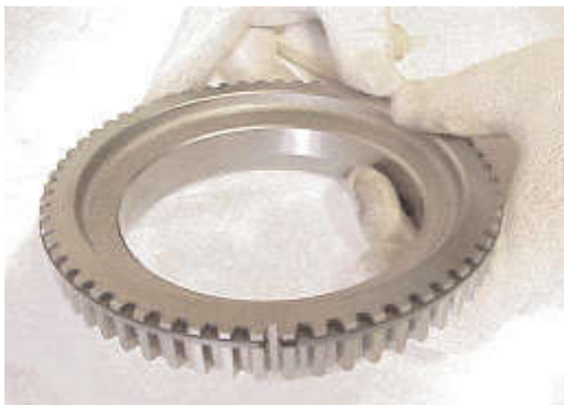
16. Install the large snap ring into the slot around the outer periphery of the low synchroniser flange.
