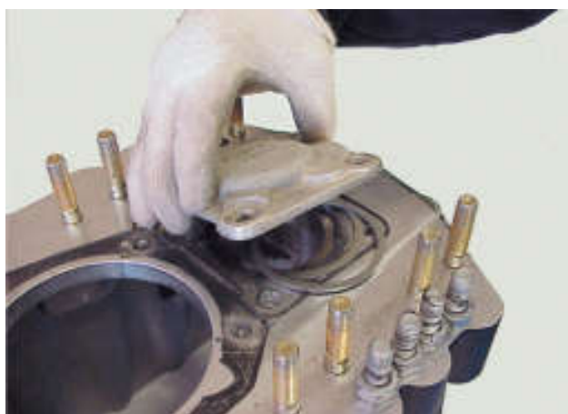
44. Remove the layshaft front bearing retaining plate and graded spacer from the front case half.
