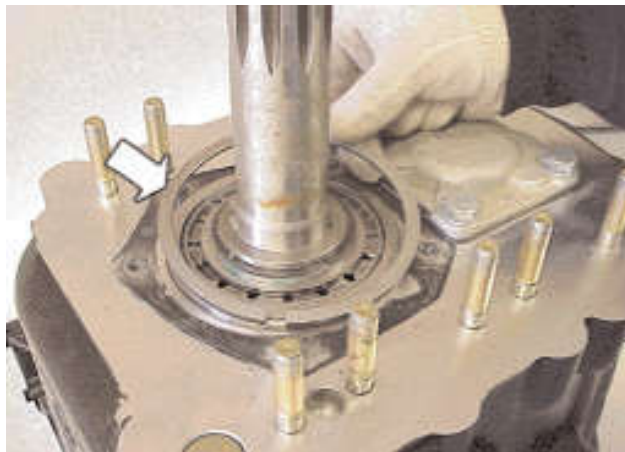
42. On overdrive models remove the input shaft bearing outer snap ring.
