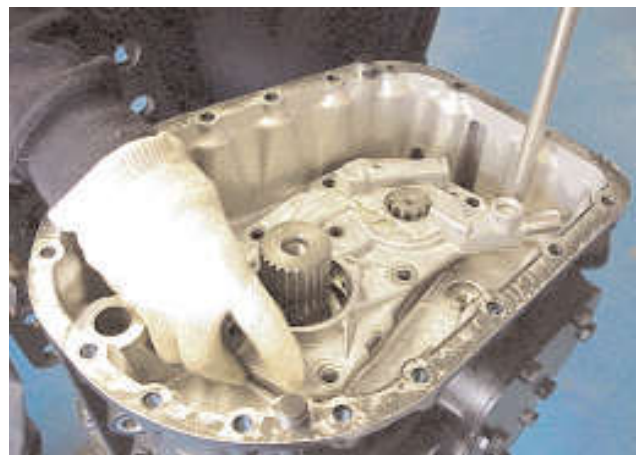
16. Using a pry bar under the lugs provided, prise the pump off the locating dowels. Lift out the pump assembly.
