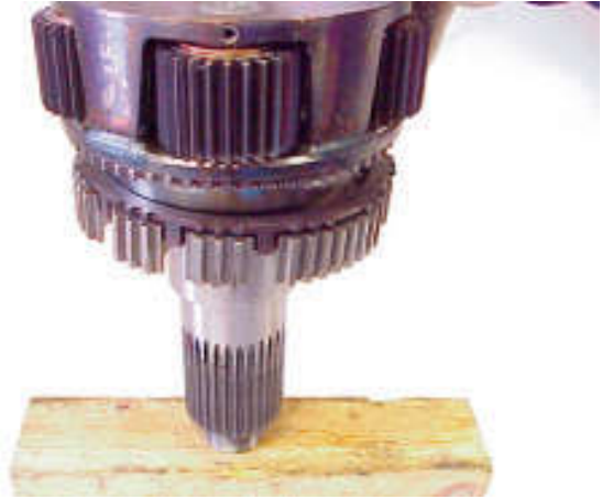
10. Invert the assembly and while restraining the hub, drop the end of the shaft onto a stout wood block to shock the hub, bearing assembly and synchroniser ring off the shaft.
