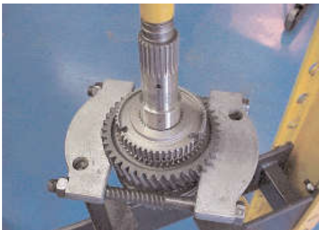
10. Assemble puller plates under the low gear and support on the press.
