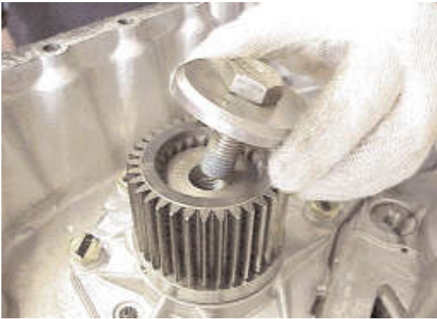
12. Using the appropriate sun gear retaining tool to lock the sun gear, unscrew and remove the sun gear retaining bolt and the special washer.
