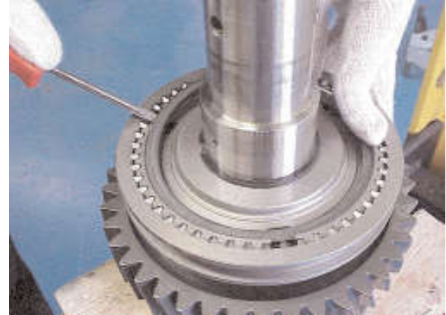
7. Remove the large internal snap ring from inside the reverse/low synchroniser hub.
