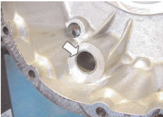
39. Replace the range change shaft bush if necessary.
