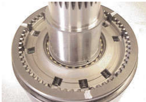
13. Remove the support lower the sleeve and ensure that the rollers are sitting in the groove of the synchroniser sleeve. Fit the rollers into the central slot of each set of grooves of the synchroniser hub.
