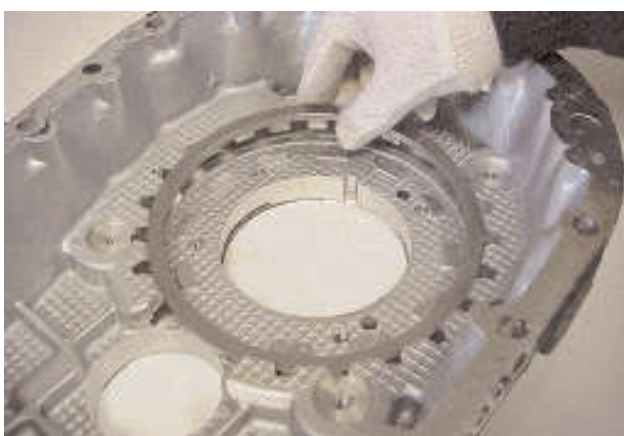
15. Support the rear case on wooden blocks and place the spacer ring into the recess in the rear case.
