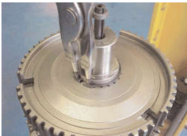
30. Fit the circlip into the mainshaft.
