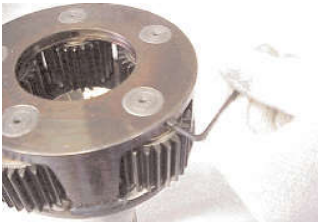
9. Ensure the threads are clean and dry and install a new locating grub screw, using thread locking sealer Loctite 270. Tighten to the correct torque and repeen with a suitable drift. Repeat sub-operations 1-9 for the remaining gears.
