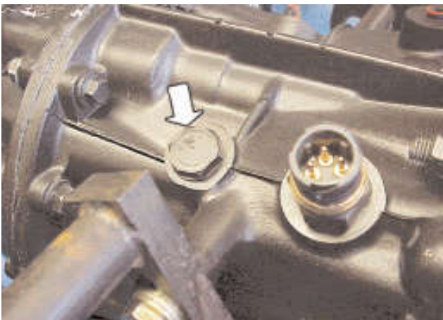
50. If fitted install the neutral switch ball and neutral switch. Alternatively install the ball, washer and plug.
