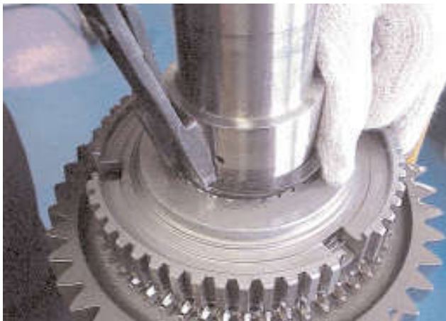
9. Remove the reverse/low synchroniser hub retaining snap ring.
