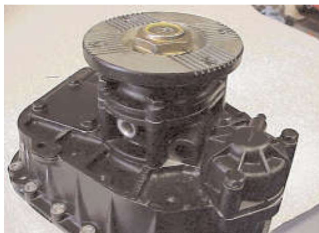
33. Apply a smear of grease to the inner periphery of the oil seal and install the output drive flange. Temporarily place a spacer against the flange and fit the nut. Tighten firmly.
