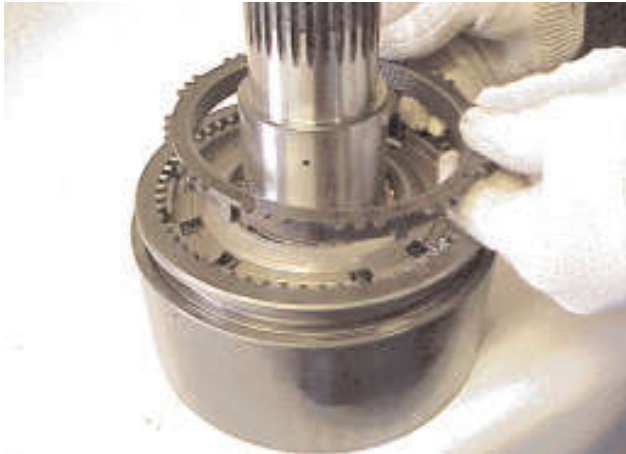
7. Lift off the synchroniser ring.
