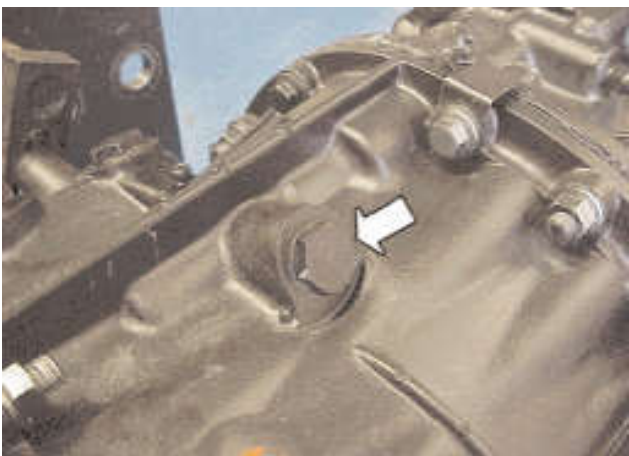
51. If fitted install the range switch ball and range switch. Alternatively install the ball, washer and plug.
