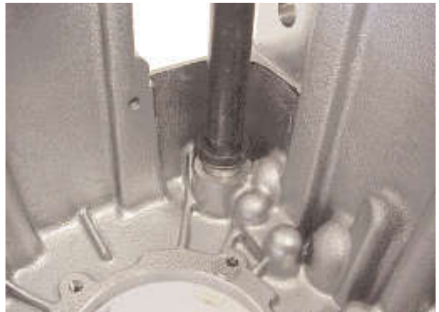
49. Fit the selector shaft bushes to the front and intermediate cases ensuring that they are fully seated.
