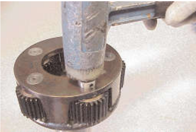
8. Ensure the locating hole in the spindle aligns with the hole in the carrier and drive the spindle into the carrier using a soft faced mallet.
