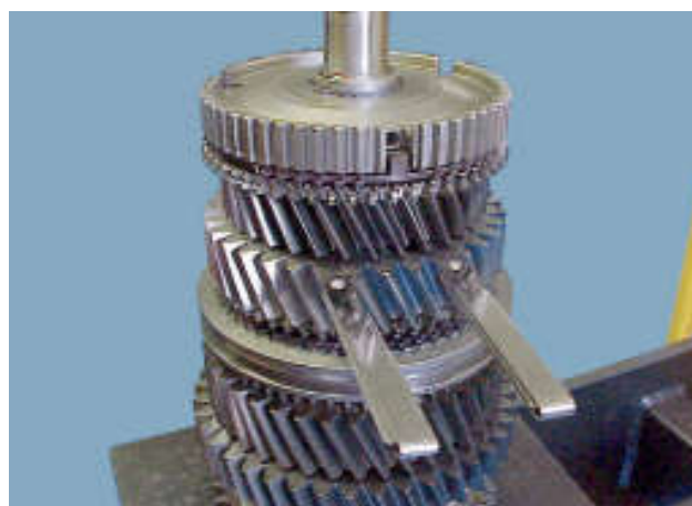
31. Check the gear end float using feeler gauges.
