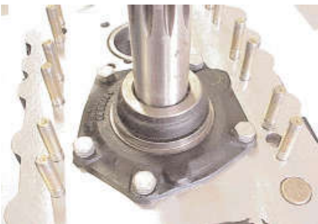
14. Lubricate the shaft seal surface and apply flange sealant to the mating face of the front cover. Install the front cover and tighten the capscrews to the correct torque.
