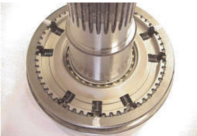
11. Install the plungers and springs in the slots and slide the annulus and sliding sleeve assembly over the planet gears, aligning the marks on the sleeve and the middle slot of each group of three in the hub
