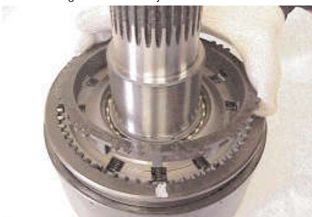
14. Place the low synchroniser ring into the synchroniser hub ensuring that the bosses on the synchroniser ring locate in slots of the synchroniser hub. Lubricate the synchroniser ring with transmission oil.
