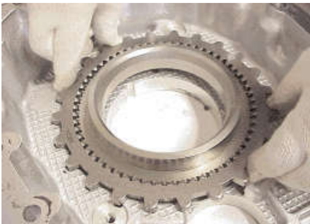
18. Place the reaction plate over the synchroniser flange splines.
