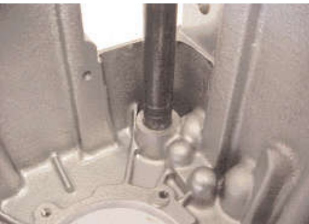
48. Apply a coating of sealant to the core plug. Drive it in, from the inside the front case, until it is flush with the front case face.
