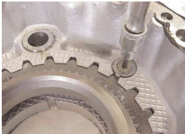
19. Install the three / four locating plates and screws. Tighten the screws to the correct torque.
