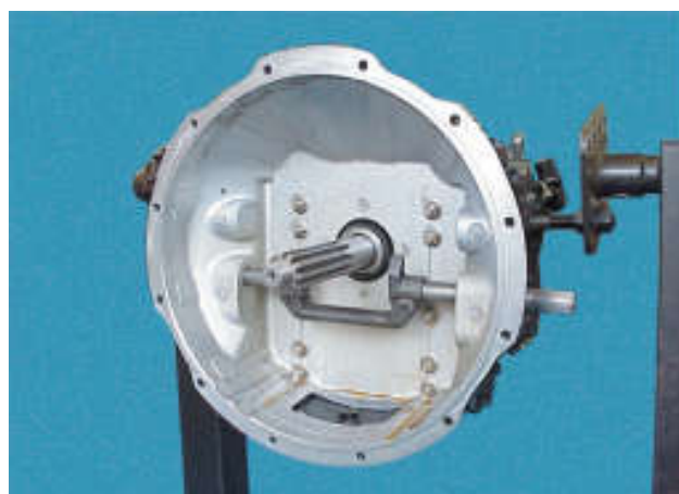
53. Refit the clutch housing assembly. Reconnect all the air lines.
