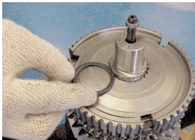
29. From the range of graded circlips select the thickest one which fits into the groove with the minimum free play.
