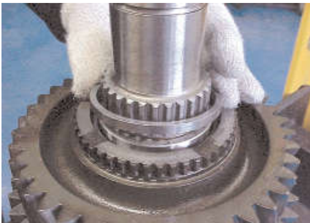
15. Install the bearing spacer ring into the gear and against the bearing.
