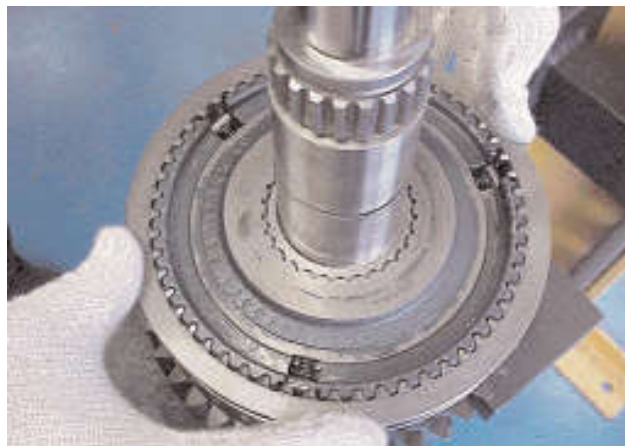
18. Assemble the three springs and plungers into the hub and install the 1st/2nd gear synchroniser sleeve and rollers as described in sub-operation 9.
