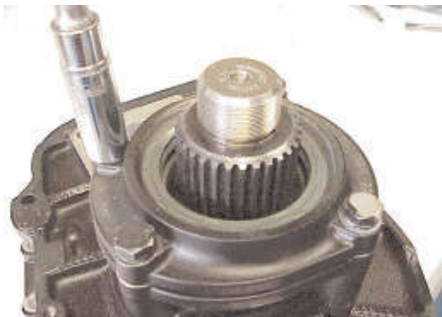
28. Apply sealant to the four capscrews and tighten to the correct torque.
