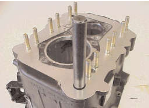
47. Drive the selector shaft bush from the front case from the outside. Drive the selector shaft bush from the intermediate case by driving the bush forwards.
