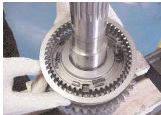
8. Slide the reverse/low gear synchroniser sleeve carefully rearwards until the three rollers are clear of the groove in the sleeve. Remove the rollers, the sleeve and the three plungers and springs from the synchroniser hub.
