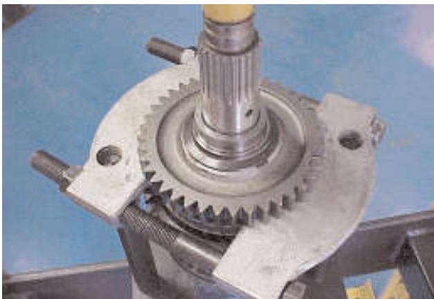
5. Invert the mainshaft assembly in the press and using suitable puller plates, under the reverse gear, remove the reverse gear and integrated bearing/thrust washer. Note: Some transmissions may be fitted with a bearing track and separate thrust washer.
