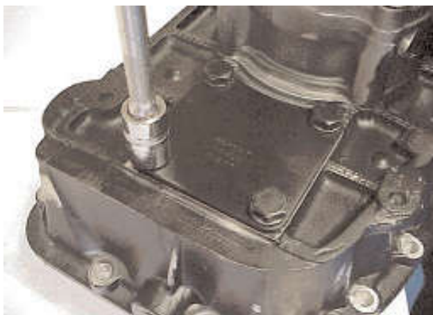
32. Apply a coating of loctite sealant and fit the rear PTO cover.
