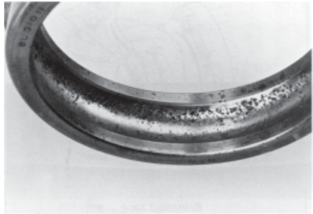
Burnt and Spalled Bearing
