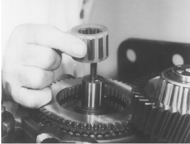
10. Lubricate and install the spigot bearing on the mainshaft.
