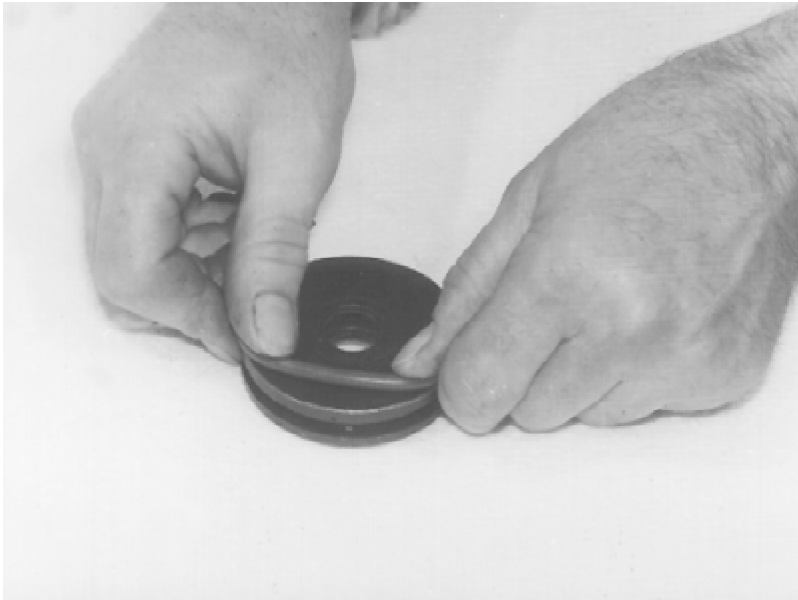
47. Apply silicone grease and fit new O-rings to the range change piston in the selector rod bore and the outer periphery.
