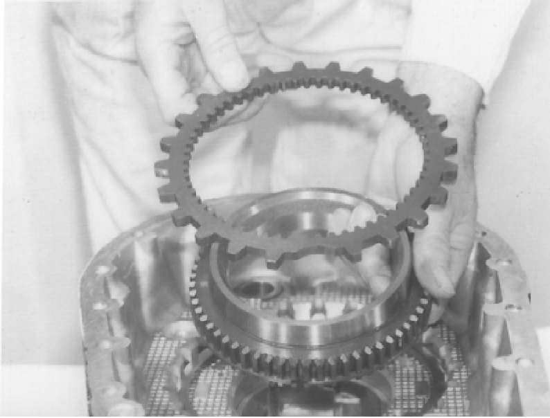
13. Lift out the reaction plate and the rear (low) synchroniser flange.
