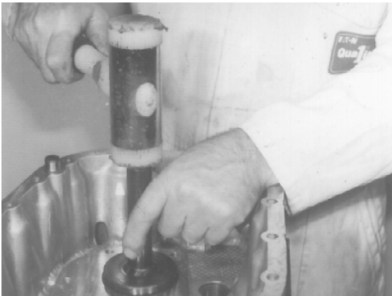
38. Drift out the layshaft rear bearing and bearing spacer (where fitted) using tool E 108-5.
