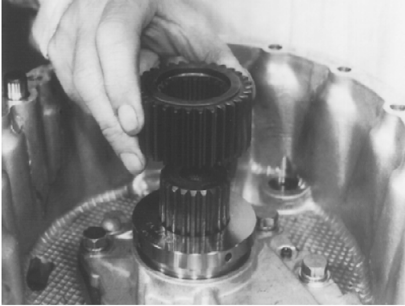
28. Install the sun gear onto the mainshaft.
