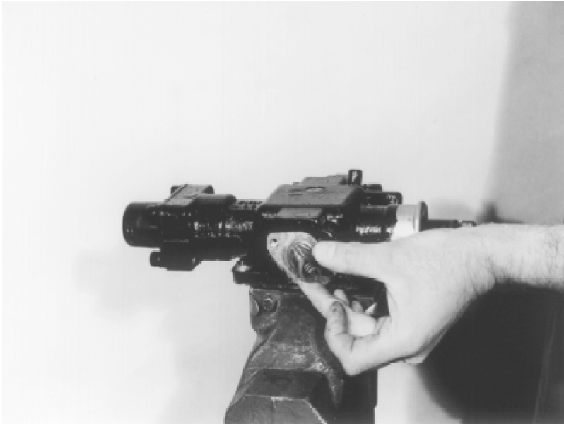
6. Remove the reverse detent plunger cover and lift out the spring and plunger.
