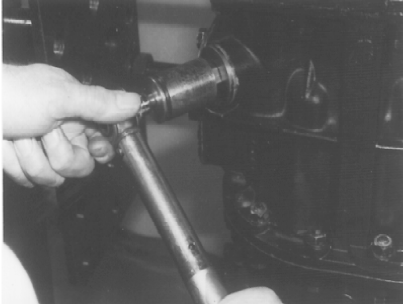
46. Tighten the strainer to the correct torque
