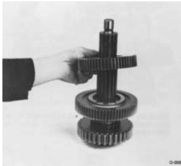
8. Remove the 2nd speed gear and washer.
