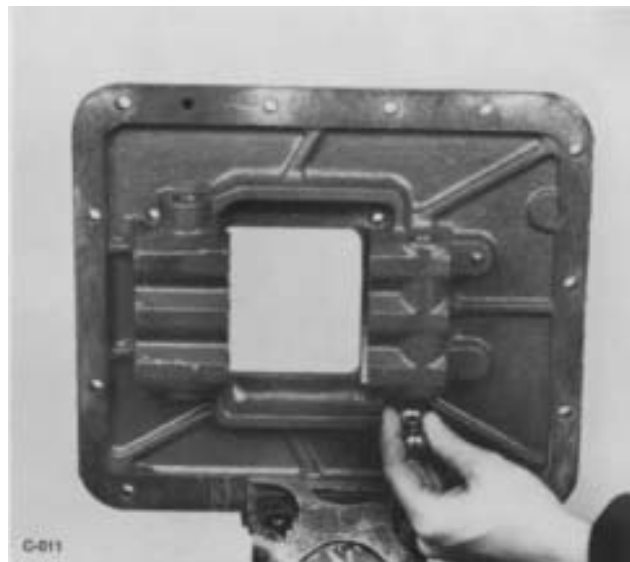
11. Remove the two interlock balls from front web.
