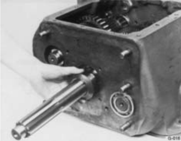
5. Remove the drive gear washer.
