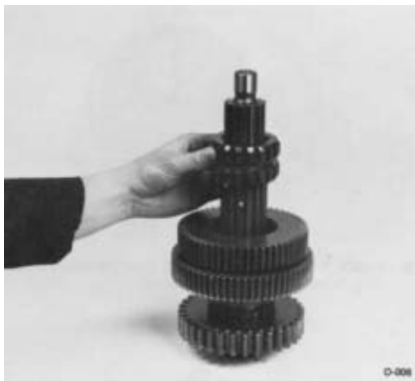
6. Remove the 2nd-3rd speed sliding clutch.
