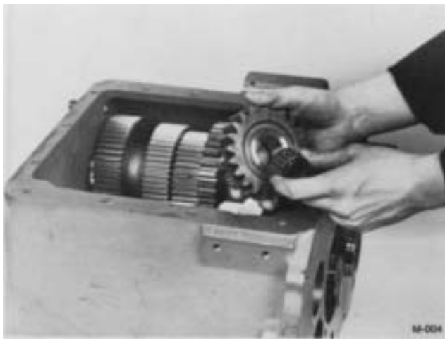
4. Remove the idler bearing from reverse idler gear.
