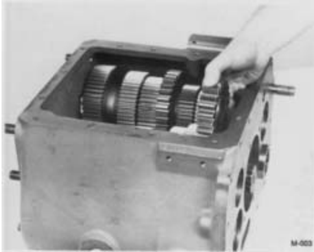
3. Remove reverse idler gear from case.
