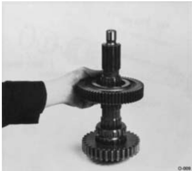
9. Remove the 1st speed gear and washer.
