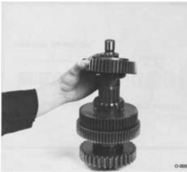
5. Remove the 3rd speed gear and washer.
