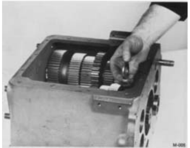
5. Remove the front idler washer from case
