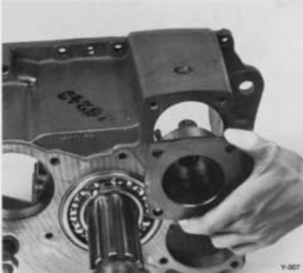
2. Remove cylinder from housing.
