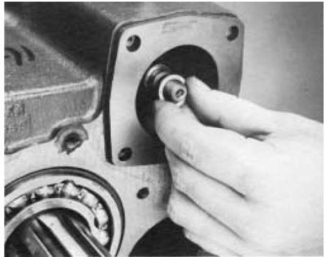
5. Remove the copper gasket from yoke bar.
