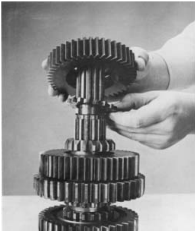
6. Remove the 2nd speed gear and tolerance washer.
