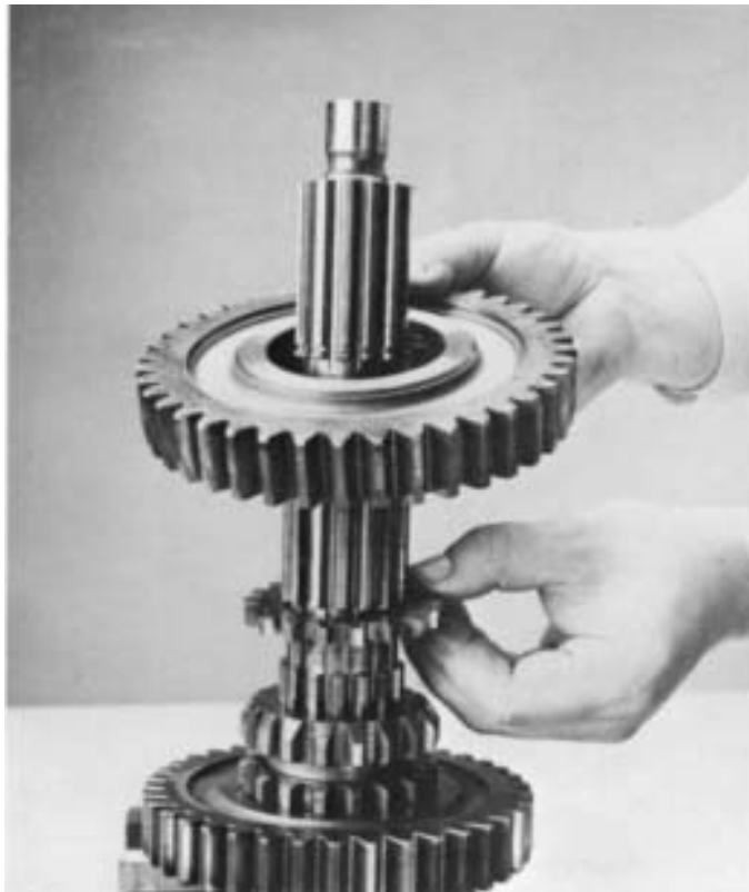
10. Remove Lo speed gear and tolerance washer.
