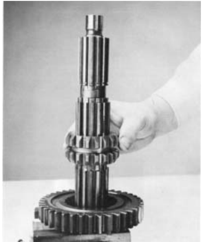
11. Remove Lo and reverse speed sliding clutch.
