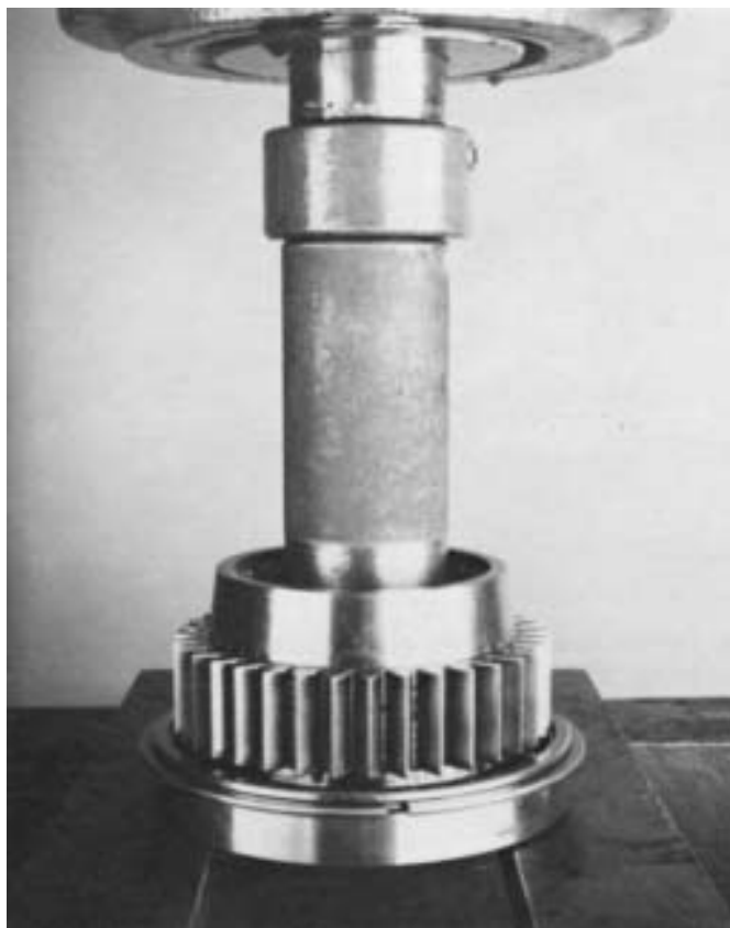
1. Press bearing on auxiliary drive gear.
