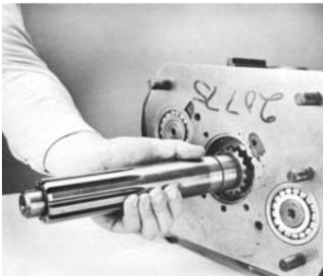
6. Pull input shaft forward and out of drive gear and case.
