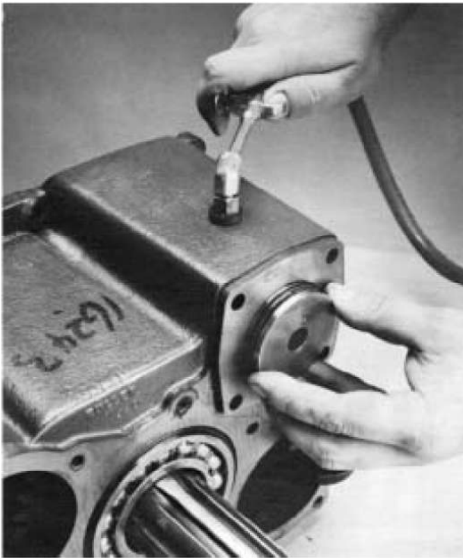
3. Use air to remove piston.
