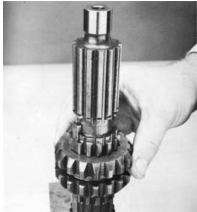
9. Install the Lo-reverse speed clutch on mainshaft, against reverse gear tolerance washer. Align slot in sliding clutch with key on mainshaft.
