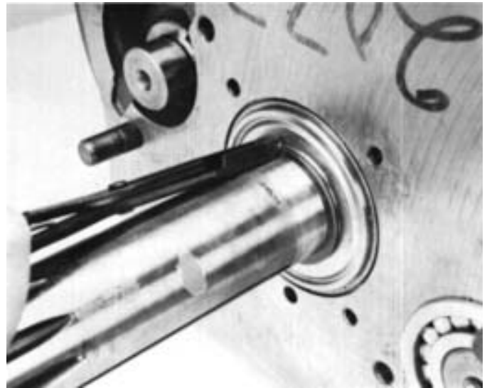
11. Install the bearing retainer snap ring.
