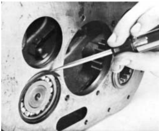
5. Install snap ring in groove in rear bore of case.
