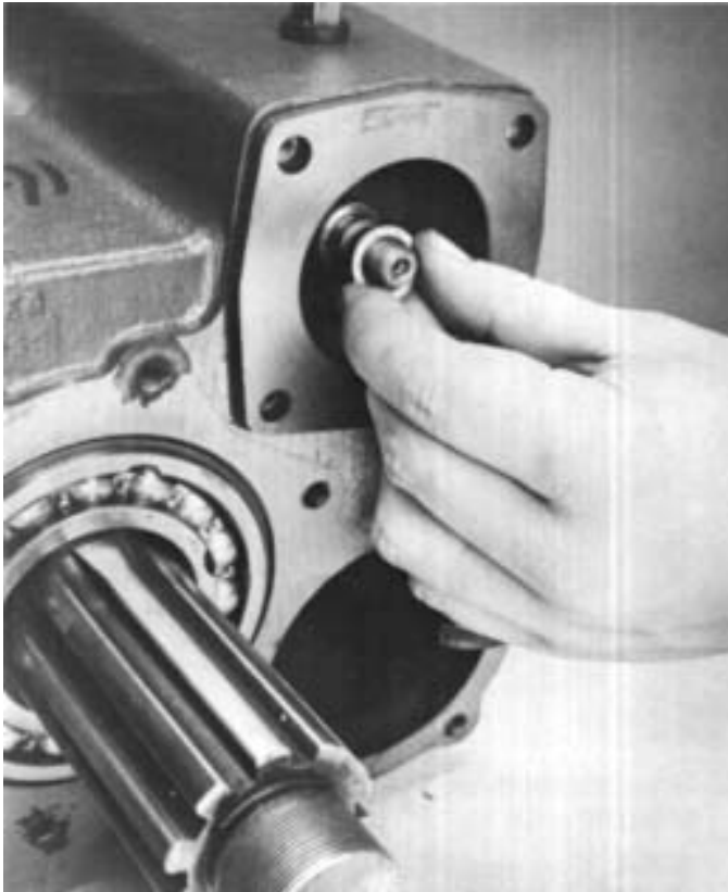
3. Install copper gasket on threaded end of yoke bar.
