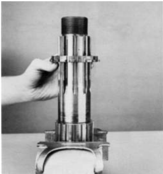
5. Remove splined spacer from output shaft.
