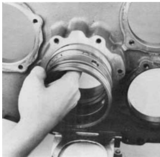
8. Remove two bearing cups and outer spacer from bore in auxiliary plate.
