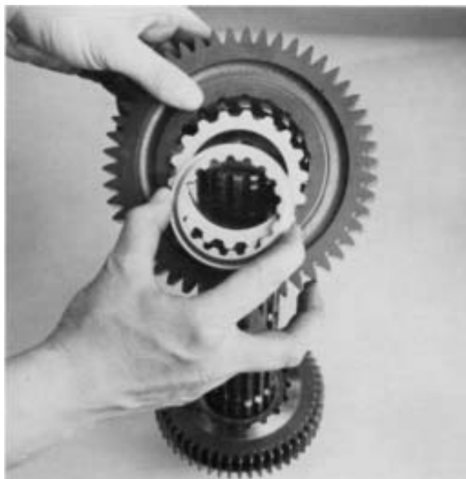
14. Lift 2nd speed gear from rear of mainshaft to remove limit washer, spacer, and gear. If necessary remove snap ring from I.D. of gear.
