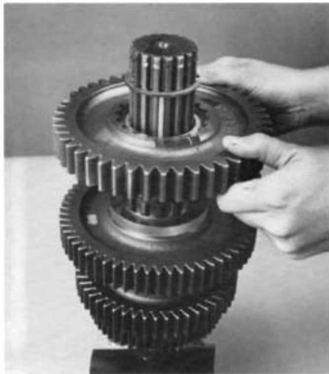
22. Install reverse gear on mainshaft, clutching teeth down and engaged with external splines of spacer.
