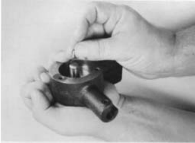
11. Remove two keys from drive shaft keyways.
