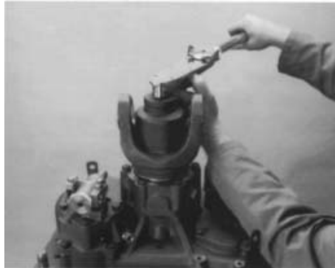
4. Complete installation process by torquing the output shaft nut to recommended torque.
