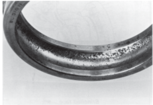
Burnt and Spalled Bearing
