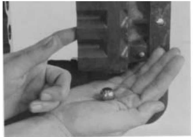
10. Remove the two interlock balls from the front web.
