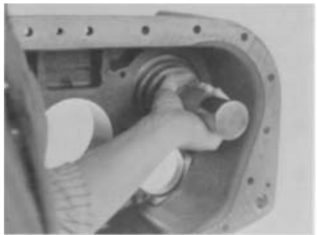
10. Drive out the two countershaft bearings.
