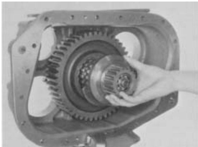
5. Install coupler, with clutching teeth to rear.
