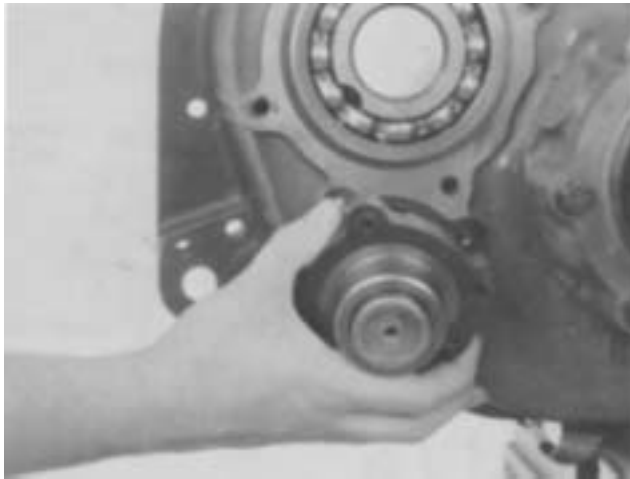
3. Remove the reduction cylinder body and yoke bar.
