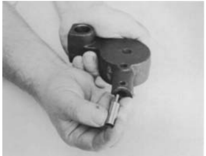
14. Remove relief valve from housing bore.
