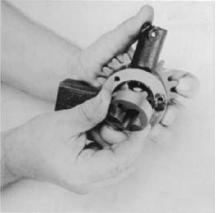
5. Remove outer oil pump element from pump.
