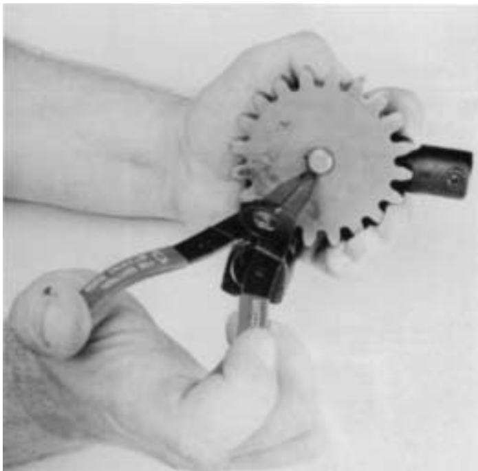
6. Remove drive gear retaining snap ring from drive shaft.
