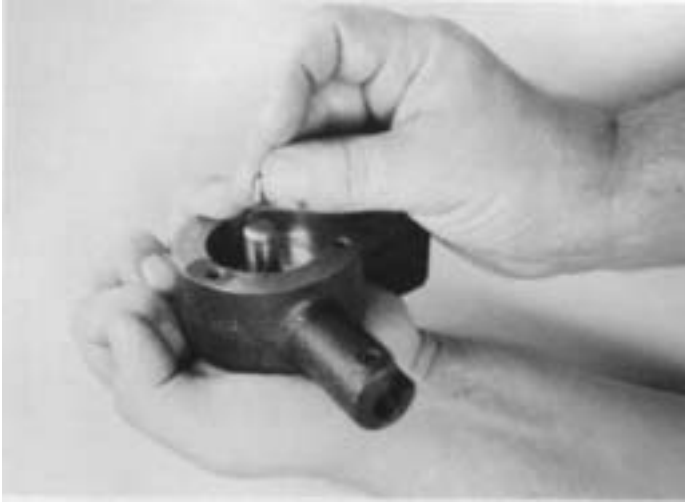
11. Remove two keys from drive shaft keyways.
