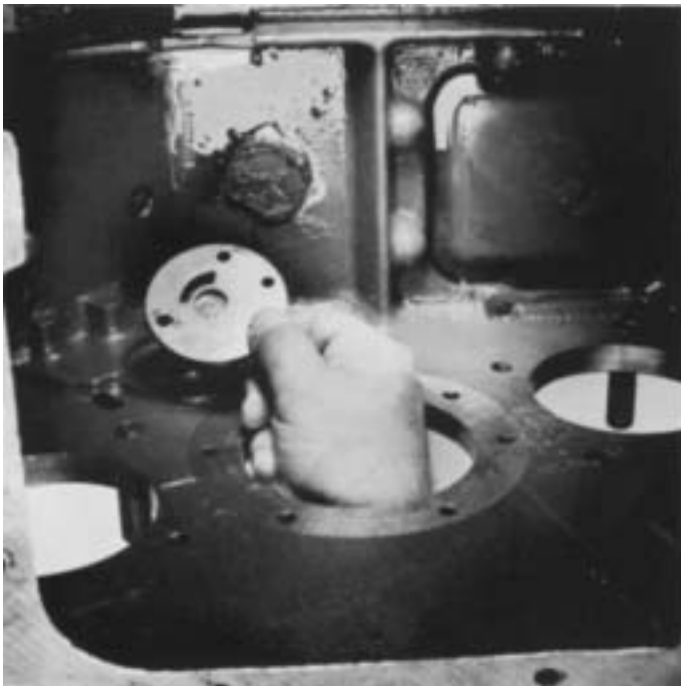
4. Remove integral oil pump retainer plate from case.
