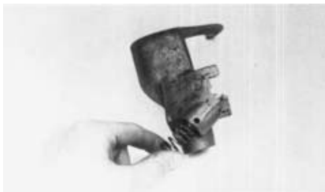
7. Install the spring in the bore and on the plunger.
