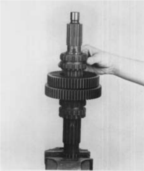
14. Remove the 2nd-3rd speed sliding clutch.
