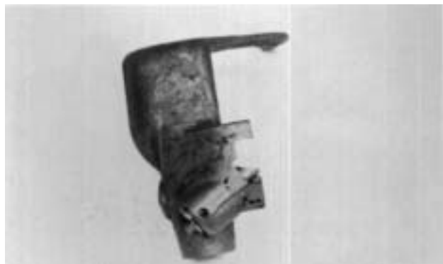
8. Partially install the plug. Use the tip of the gear shift lever to push the plunger back into the bore to compress the spring. Tighten the plug fully and then back off 1/2 - 1 1/2 turns. Stake the plug threads in the hole.
