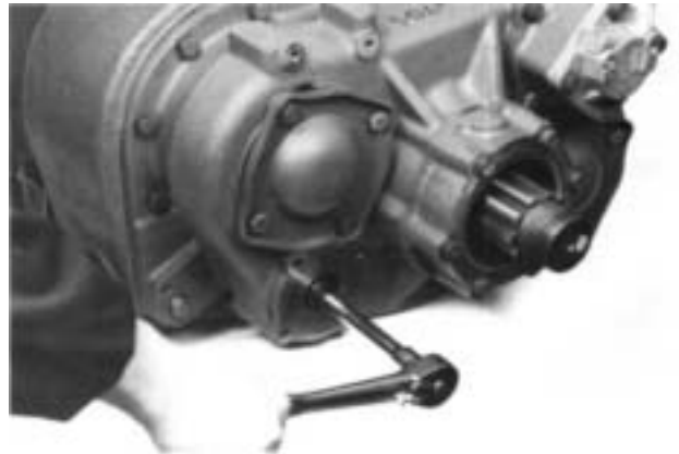
9. Install the elastic stop nut on the shaft.
