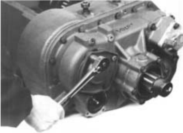
5. Install the rear bearing covers.
