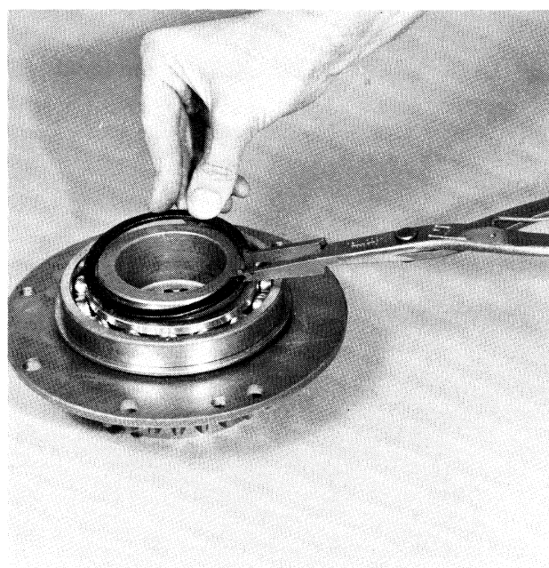
4. Remove the snap ring from the shoulder of the drive gear; press the retainer ring and bearing from gear.
