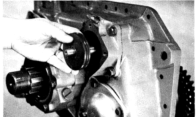
3. Push the yoke bar to the rear and out of the housing. Remove the piston from the yoke bar and if necessary, remove the O-rings from the ID and OD of the piston.
