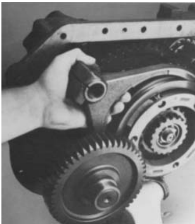
5. Remove range yoke from sliding clutch of syn- chronizer assembly.
