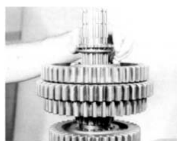
18. Install the spacer, flat surface down.
