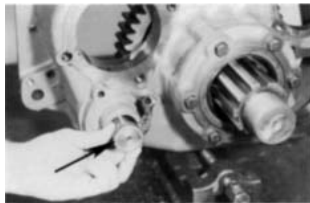
3. Push the yoke bar to the rear and remove from the housing. If necessary, remove the O-ring from the bar, (arrow).
