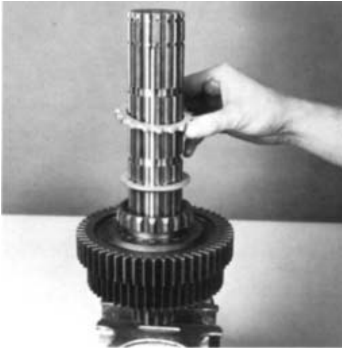
12. Install the spacer on shaft against washer.
