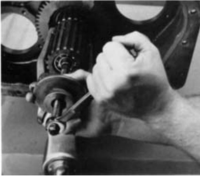
5. Remove range mainshaft with jaw puller.
